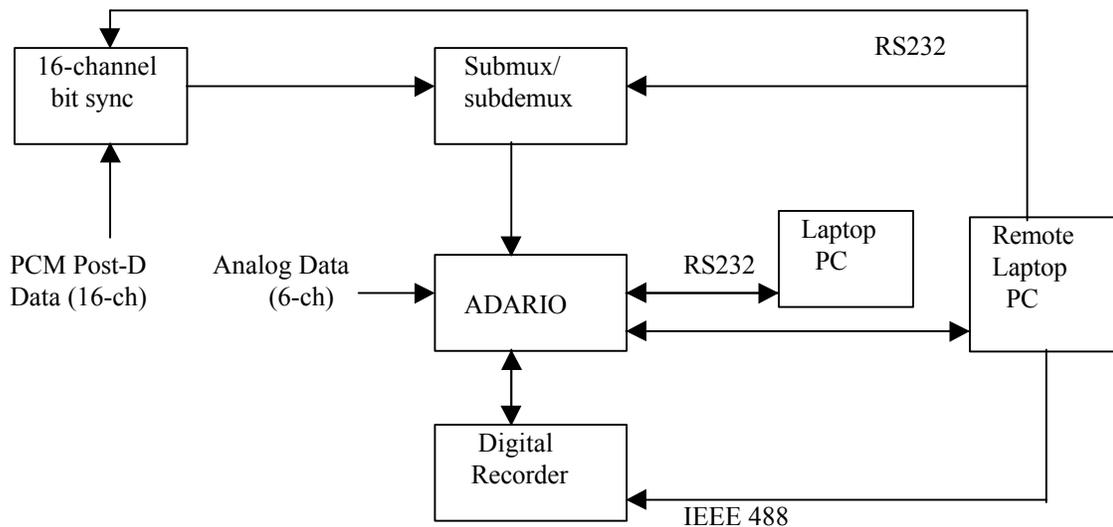
**Figure 1: HDDR System Block Diagram**
