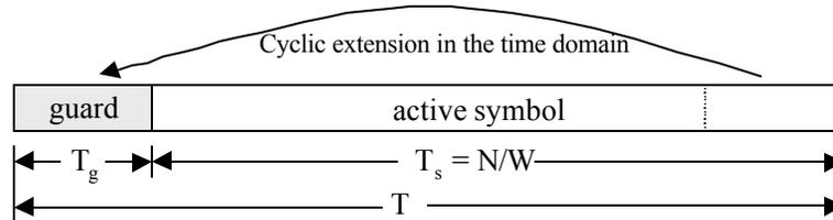
**Figure (2)** Method for implementing the guard band, creating a cyclic extension of the OFDM symbol.
