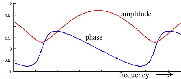
**Figure (4)** Frequency response of null with  $\tau = 50$  ns,  $\Gamma=0.7e^{j\pi/2}$ .
