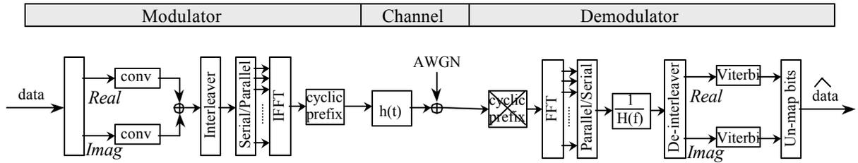
**Figure (3)** Block diagram for OFDM modulation and demodulation using the FFT.
