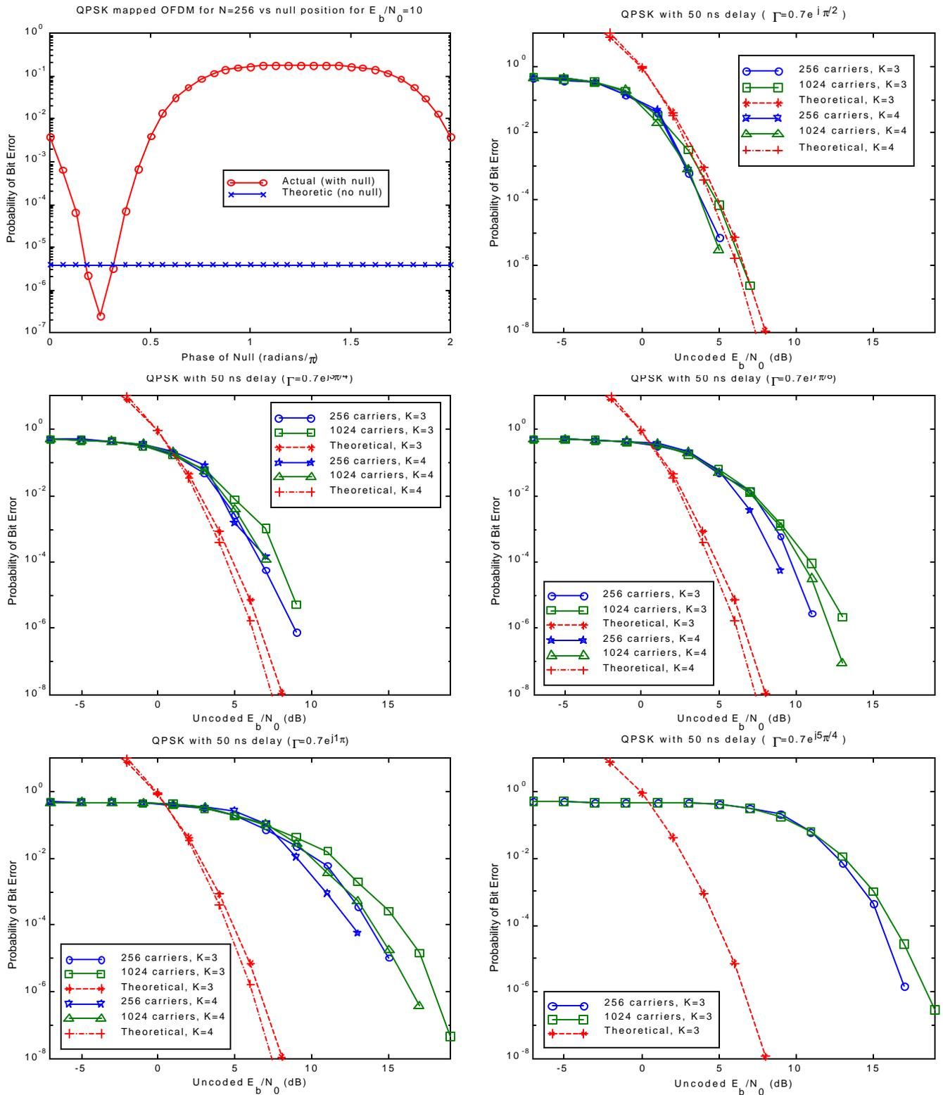
**Figure (5)** The effects of the phase of the null on telemetry transmission. UL: Probability of bit error as a function of null phase  $\mathbf{g}$  for fixed  $E_b/N_0 = 10$  dB and no coding. Clockwise from upper right: Performance of theoretical rate  $\frac{1}{2}$  convolutionally encoded QPSK in the AWGN channel without fading vs. COFDM on multipath fading channel with null phase  $\mathbf{g} = \pi/2, 7\pi/8, 5\pi/4, \pi, 3\pi/4$ .
