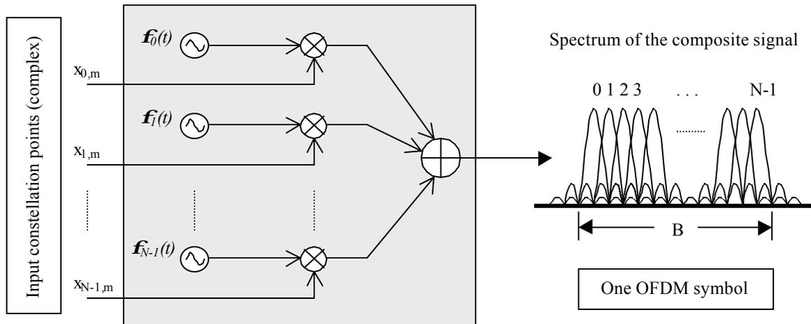
**Figure (1)** Conceptual method of OFDM symbol creation. All of the operations in the shaded box can be replaced with the inverse DFT.
