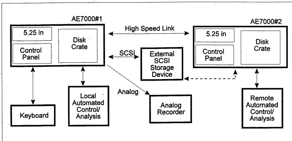
Figure 7: AE7000 Typical Data Flows
