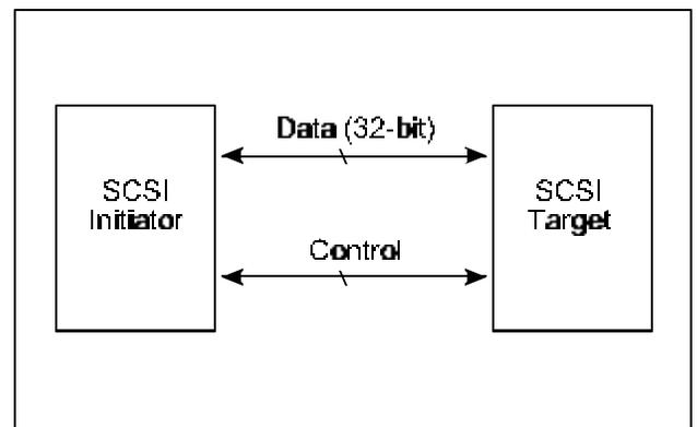
Figure 5: SCSI Data/Control Interface (fast/wide implementation)
