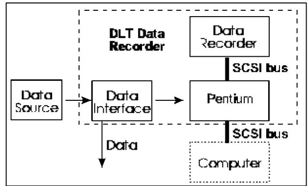
Figure 2. DLT Recorder Architecture
