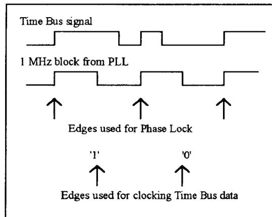
Fig. 4. Time bus decoding.
