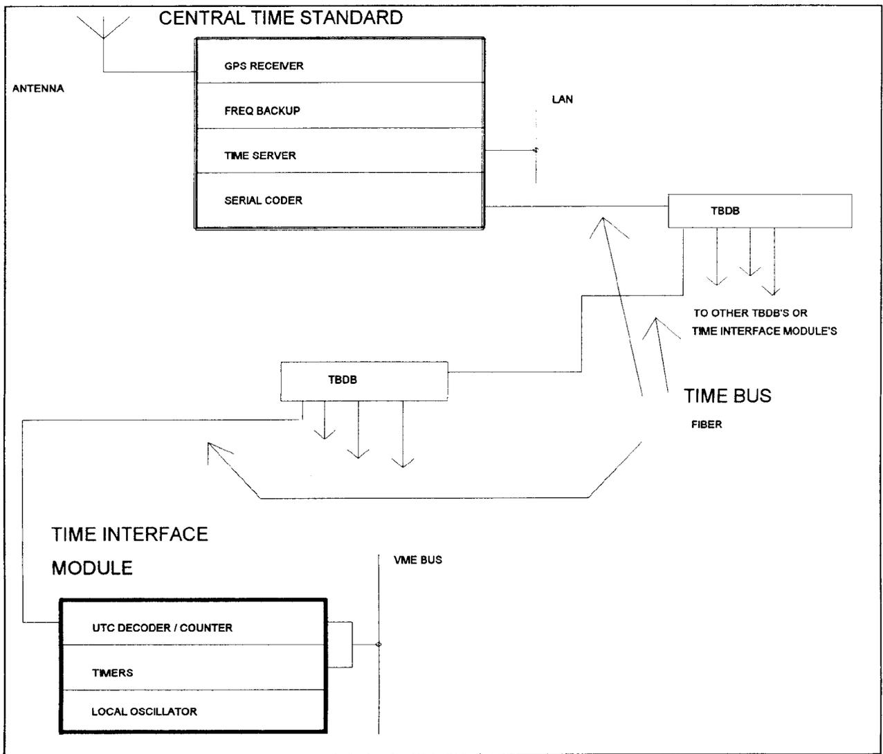
Fig. 1. TRS block diagram.
