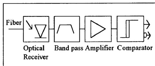
Fig. 2 TBDB receiver board, block diagram.
