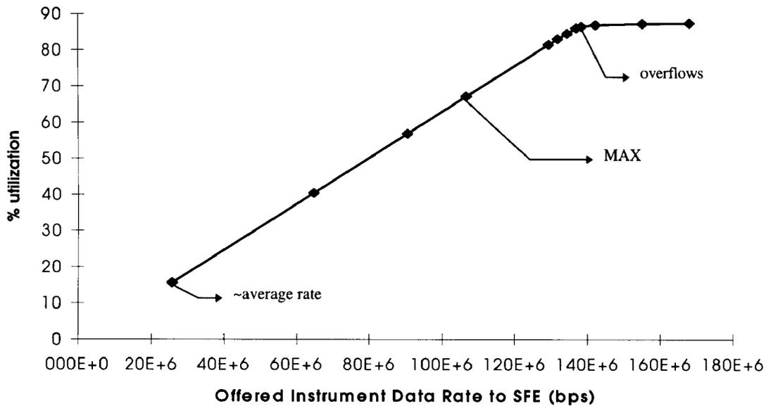
Figure 6: Loading on the PSB as a Function of Aggregate Instrument Data Rate
