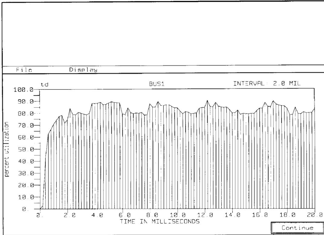
Figure 5: Loading on the HPM1 Local Bus at the Maximum Allocated Instrument Data Rates (NETWORK II.5 generated)
