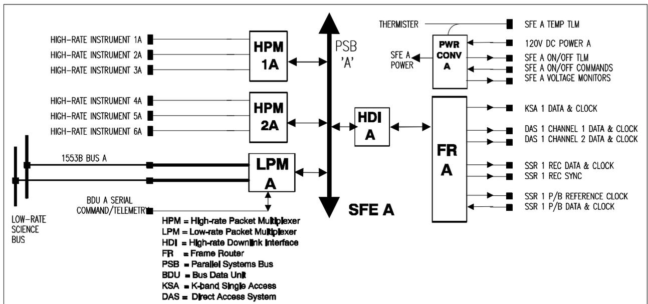
Figure 1: Block Diagram of the SFE
