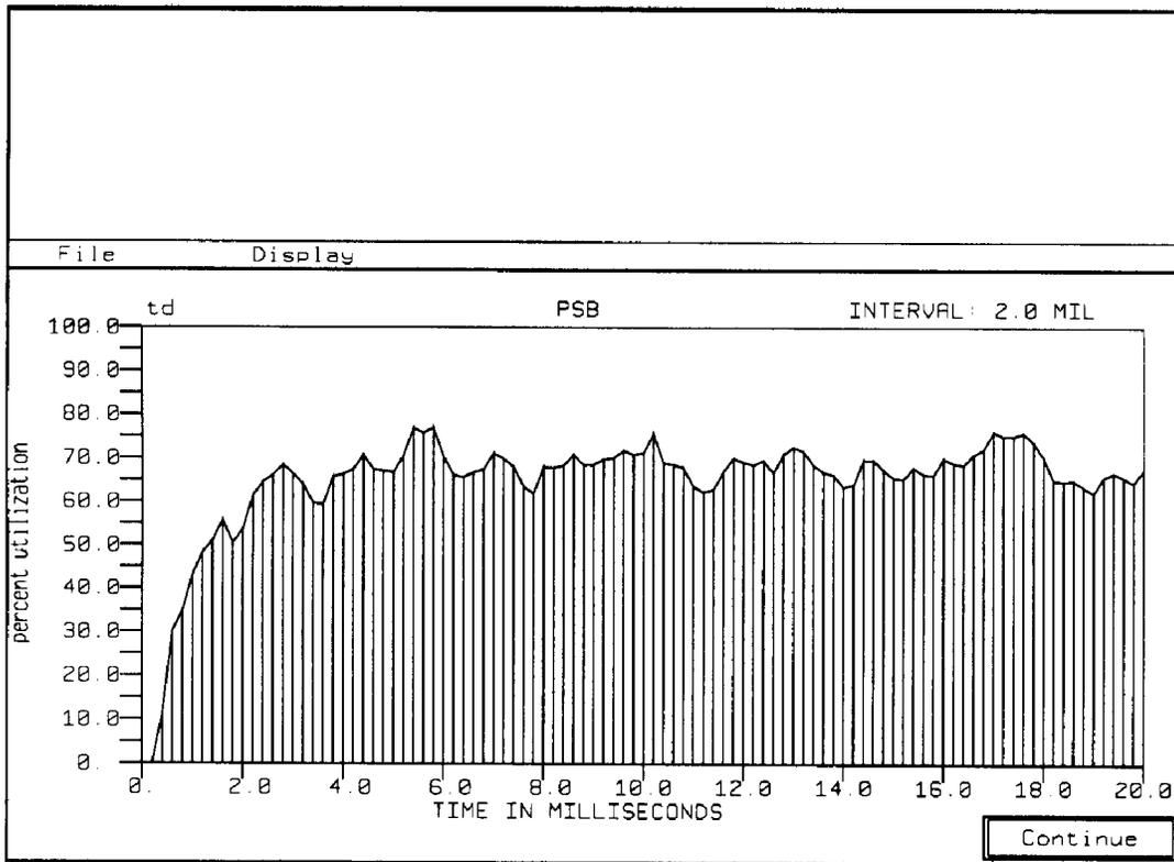
Figure 4: Loading on the PSB at the Maximum Allocated Instrument Data Rates (NETWORK II.5 generated)
