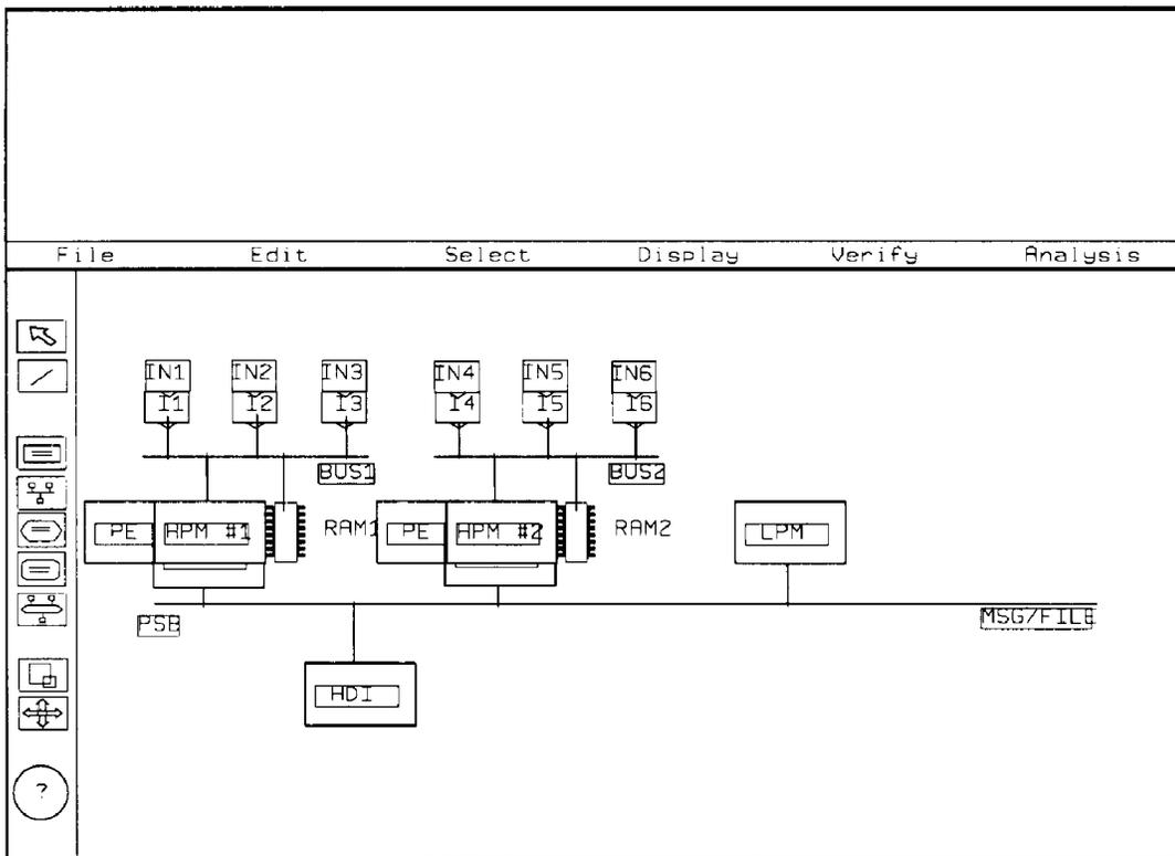
Figure 3: Simulation Hardware Block Diagram (NETWORK II.5 generated)
