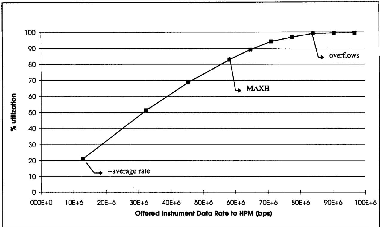
Figure 7: Loading on the HPM Local Bus as a Function of Instrument Data Rate
