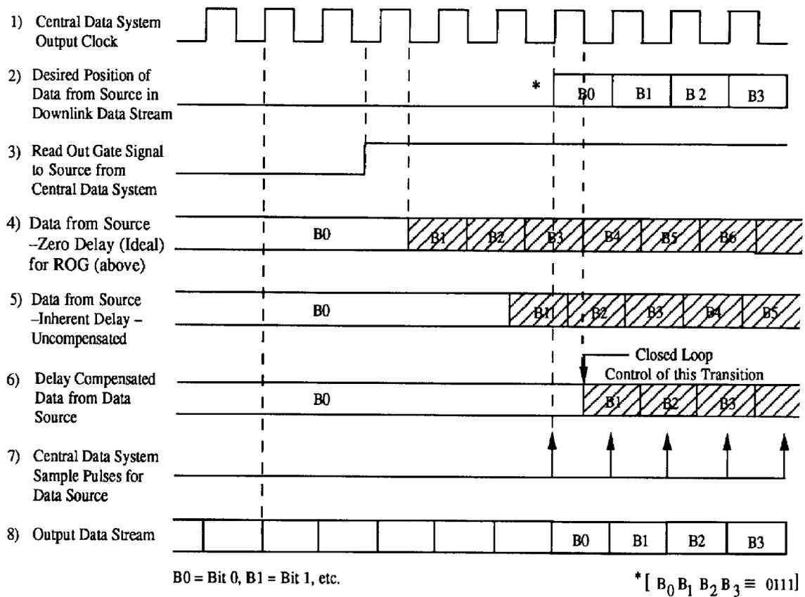
Figure 4. Delay Compensation Timing for One Data Source
