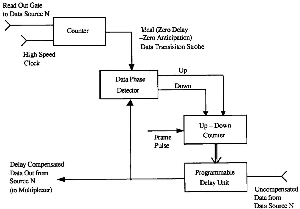
Figure 5. High Rate Data Delay Compensation Network
