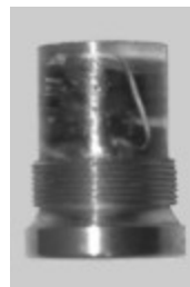
Figure 15. Encapsulated Tracer Well Assembly
