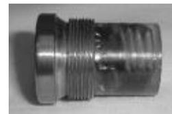
Figure 4b. Instrumented tracer-well section.
