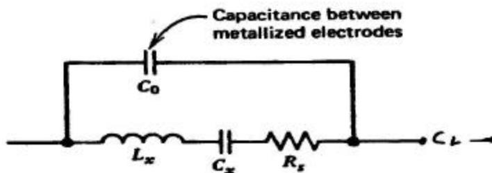
**FIG. 3** Equivalent circuit for a quartz crystal near fundamental resonance.
