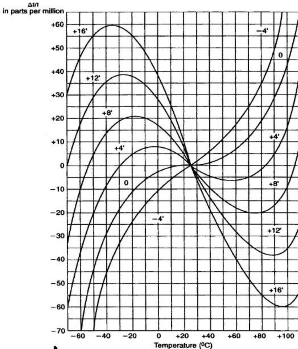
FIG. 5 Temperature characteristics of AT-cut crystals versus slight changes in cut-angle.
