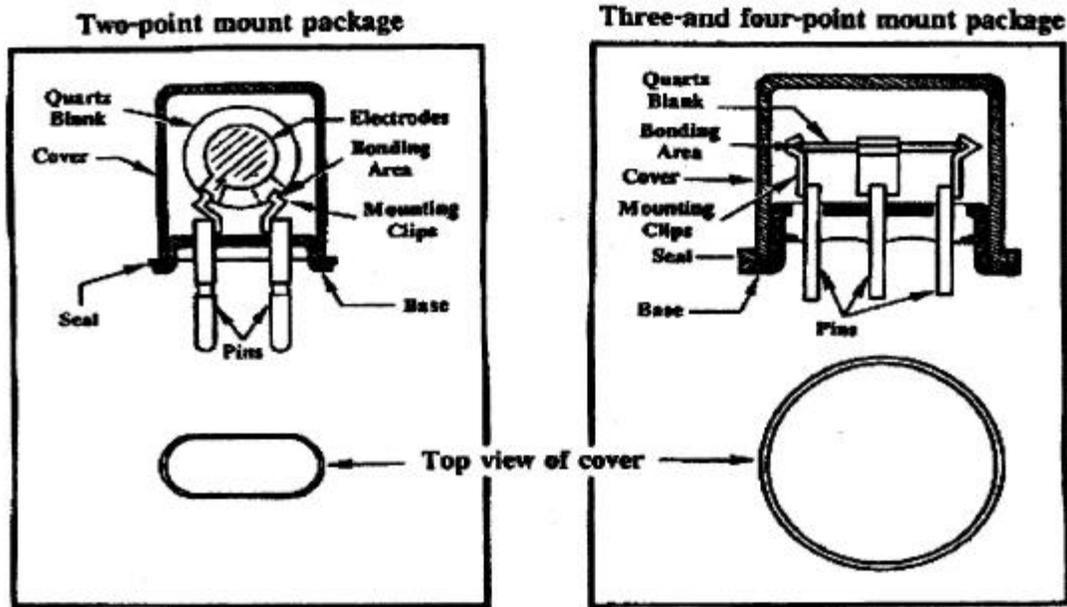
FIG. 4 Typical construction of AT-cut and SC-cut crystals.
