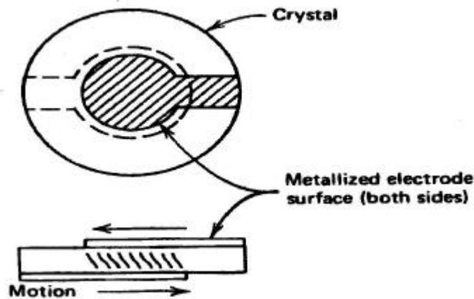
FIG. 2 Shear motion of an AT-cut crystal at fundamental resonance.
