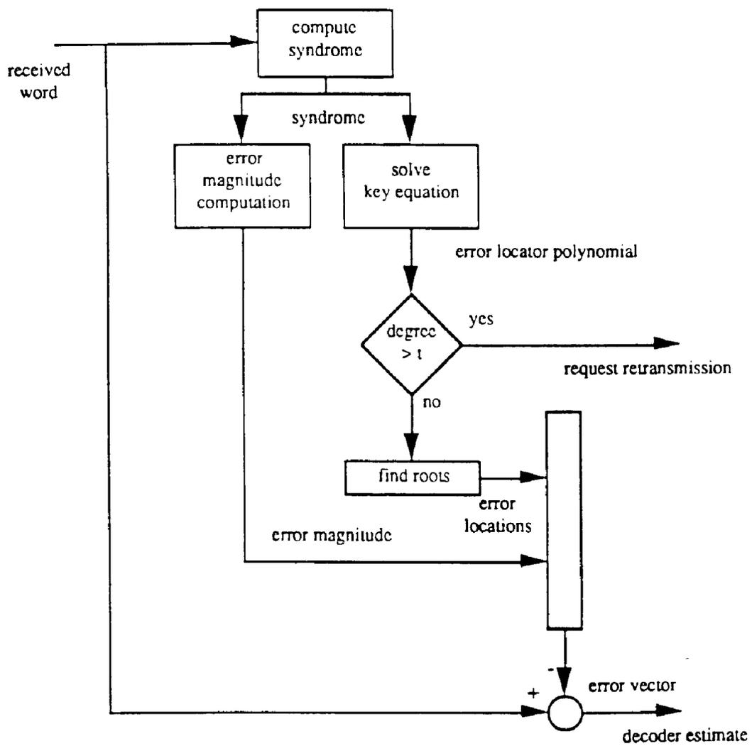
Figure 1: Modification of the Algebraic FEC Decoder
