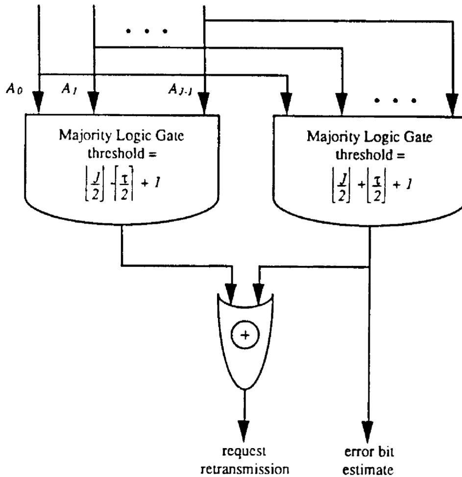
Figure 2: Modification of the Majority Logic Estimation Circuitry
