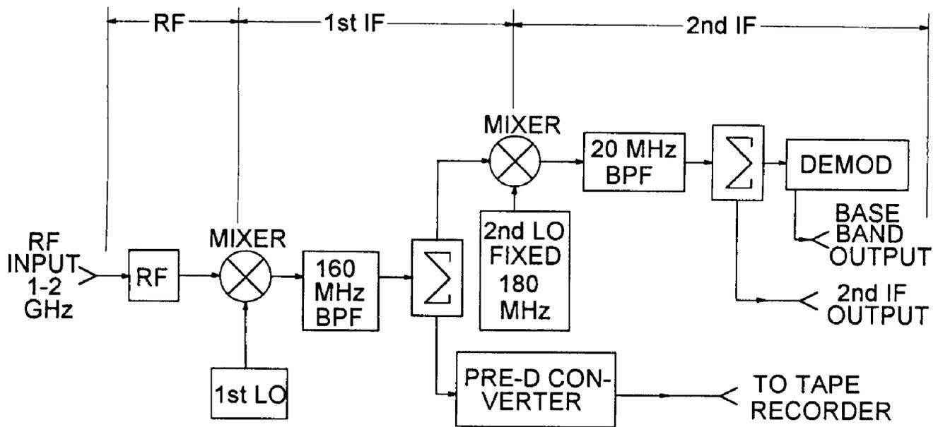
Figure 1-1. Receiver/Pre-D Converter, Block Diagram
