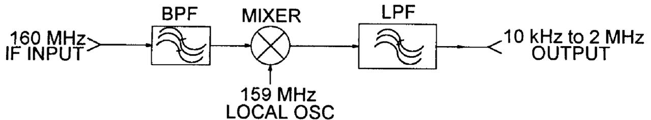
Figure 1-2. Simple Converter, Block Diagram
