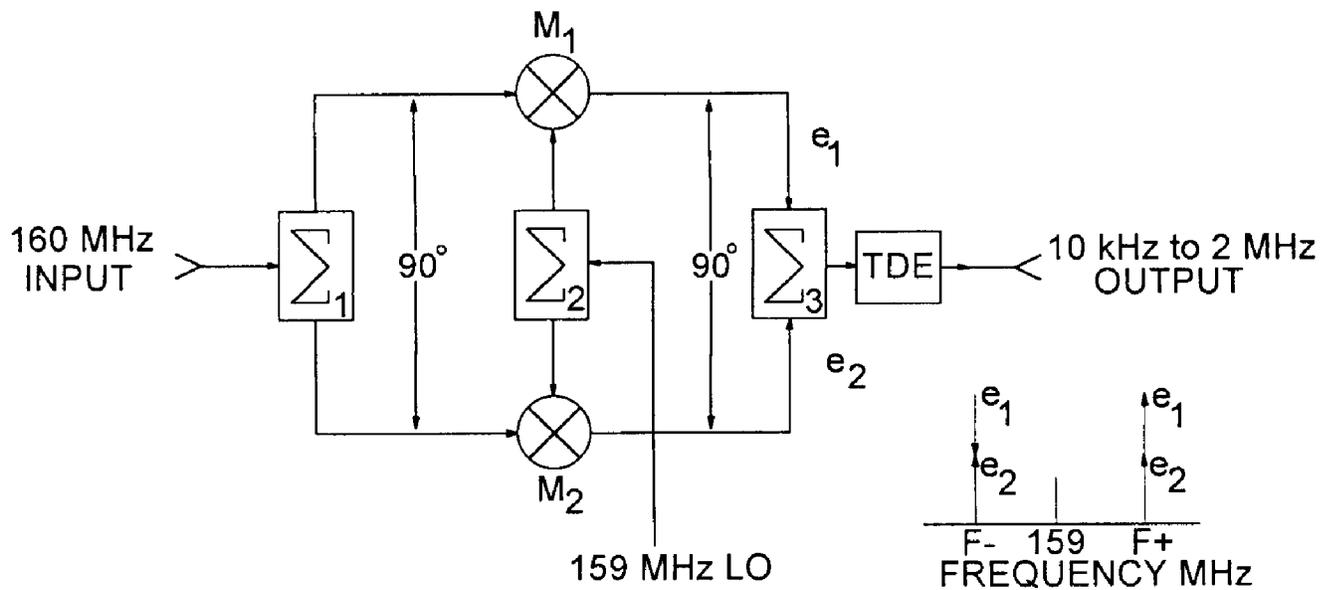
Figure 1-3. Typical Imageless Mixer, Block Diagram
