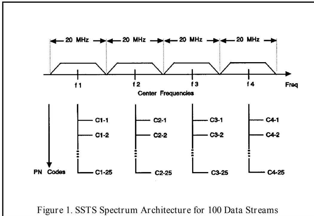
illustrate an SSTS using the CDMA technique does not interfere with the NBTR operating simultaneously in the same band on a typical test range.
