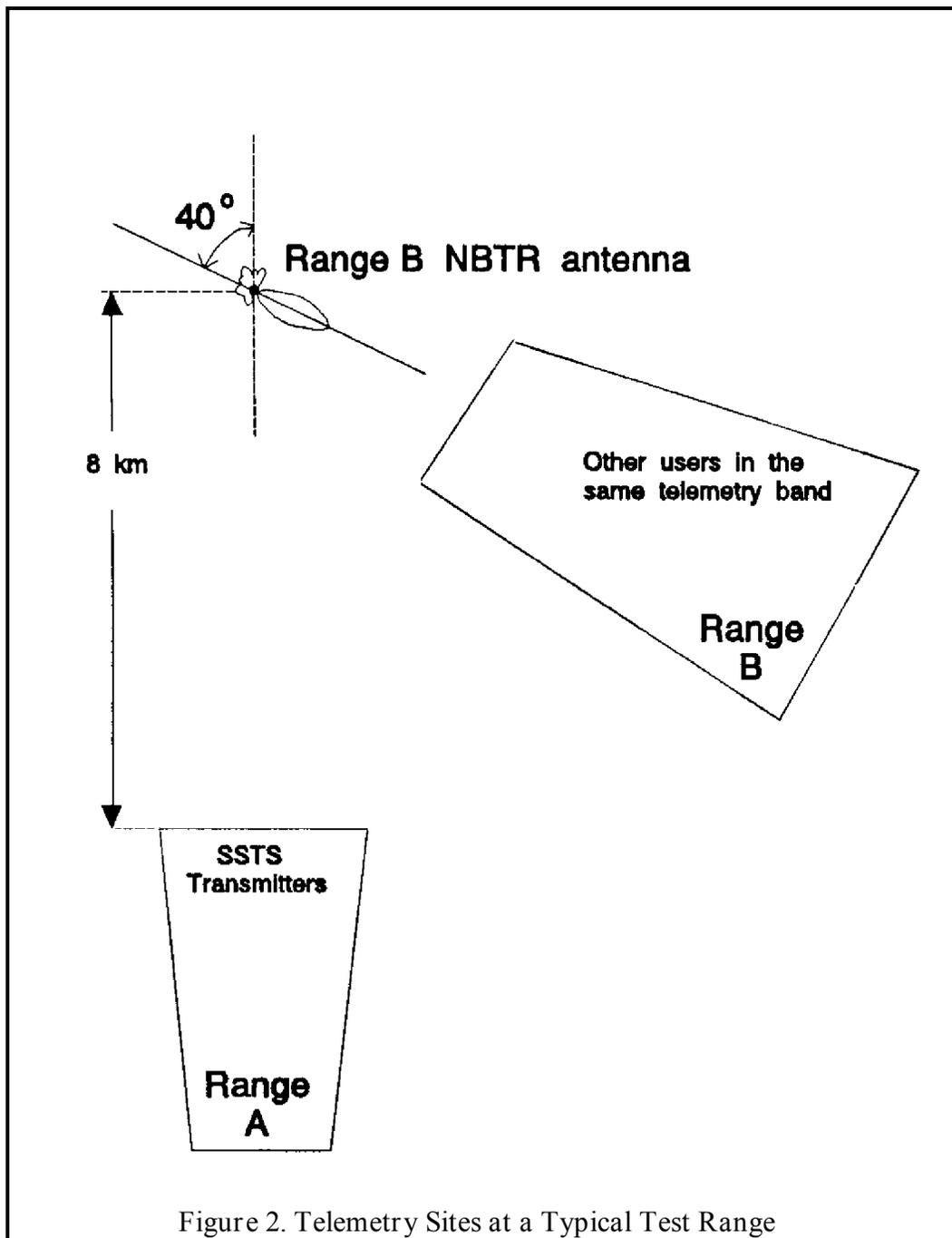
Figure 2. Telemetry Sites at a Typical Test Range
