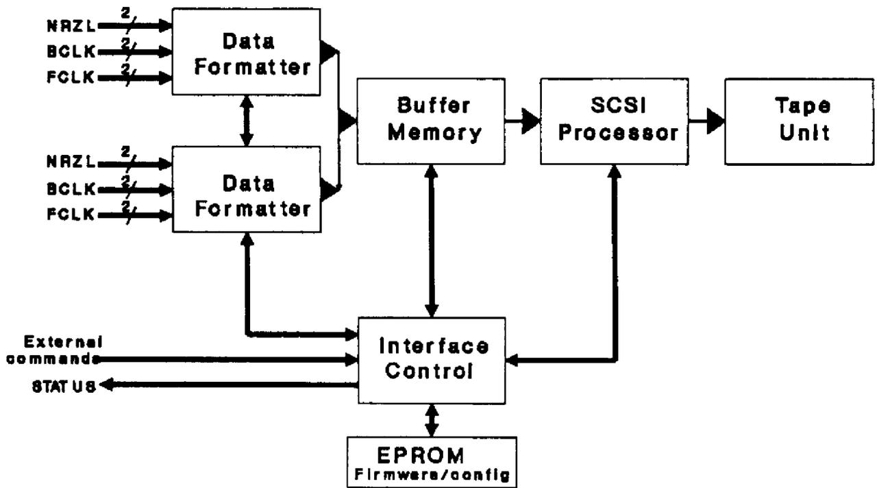
Figure 1. ATD-800 Functional block diagram
