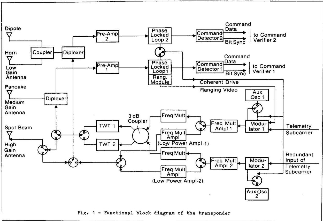
Fig. 1 - Functional block diagram of the transponder
