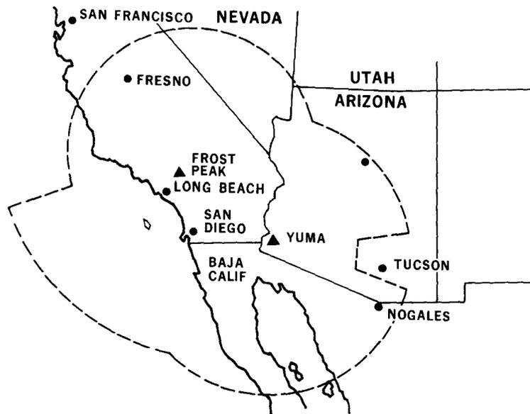
**FIGURE 7. TELEMETRY/MICROWAVE COVERAGE - AIRCRAFT AT 30,000 FT**
