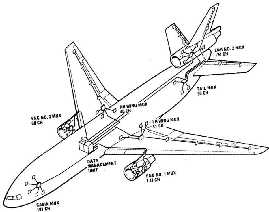
**FIGURE 6. REMOTE MULTIPLEXER DATA SYSTEM INSTALLATION**
