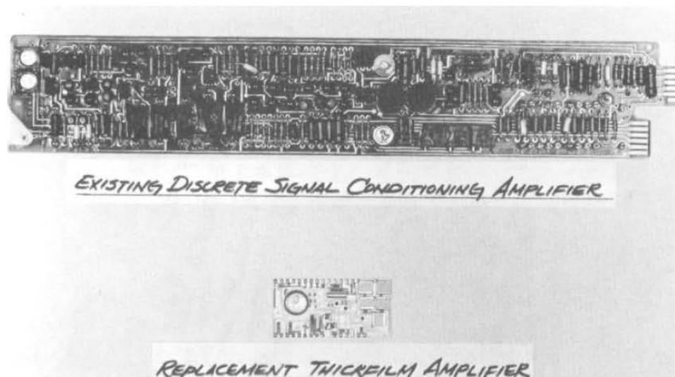
**FIGURE 3. SIGNAL CONDITIONING AMPLIFIERS**
