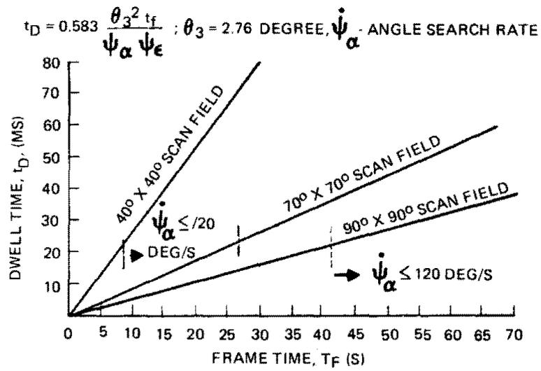
**Figure 9. Target Dwell Time in Search Beam Width**
