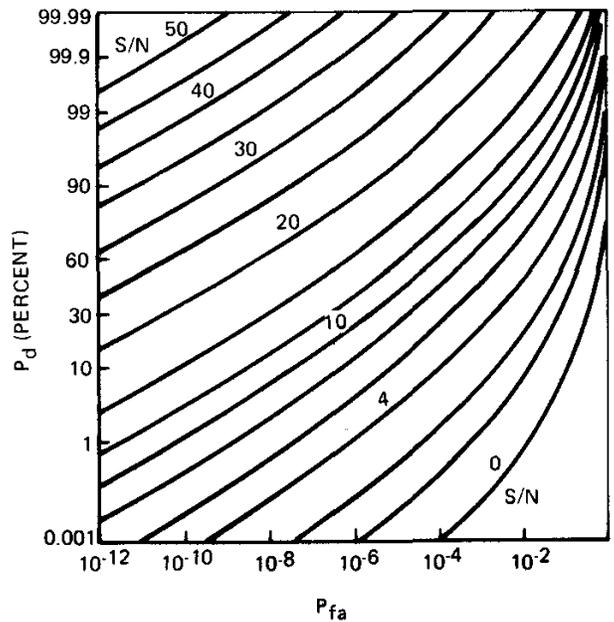
**Figure 12. Probability of Detection of a Steady-Target Versus Probability of False Alarm**
