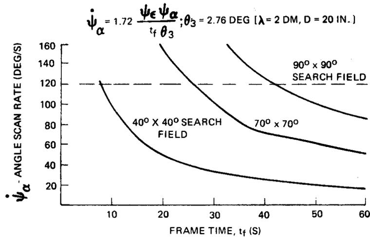
Figure 8. Required Angle Scan Rate
