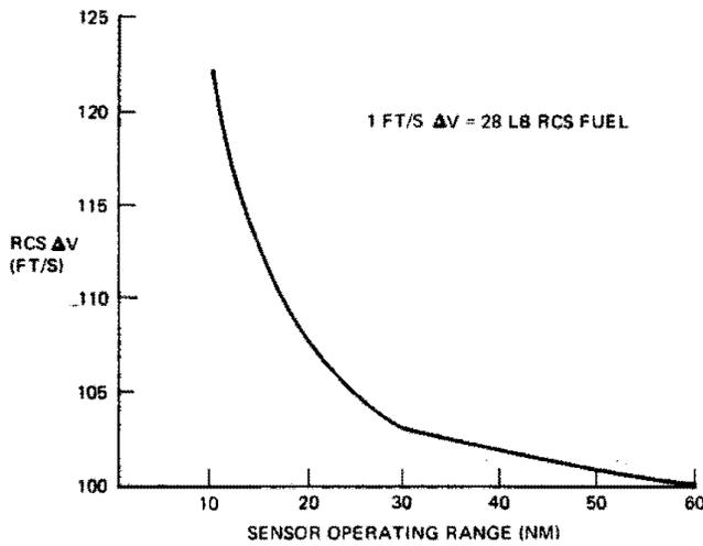
**Figure 4. Long-Range Rendezvous RCS  $\Delta V$  Required as a Function of Sensor Operating Range**
