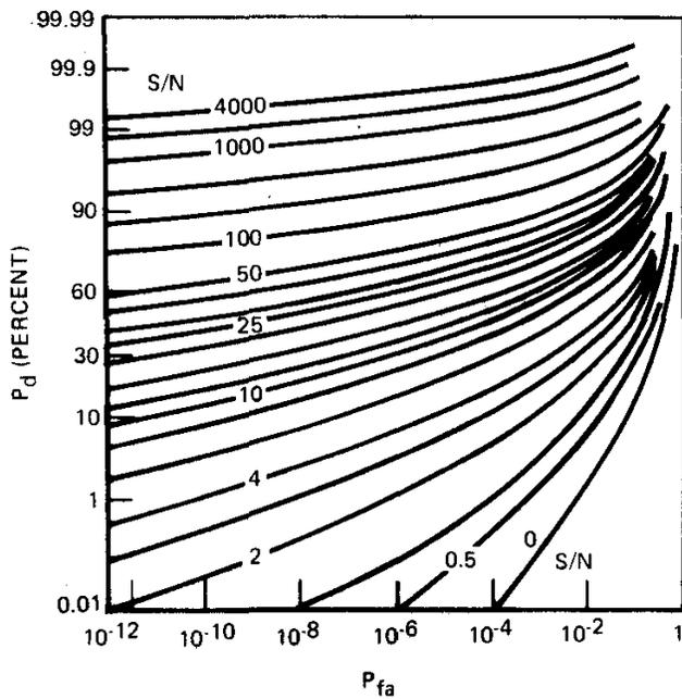
**Figure 11. Probability of Detection Versus False Alarm Probability for a Swerling Case I Fluctuating Target**
