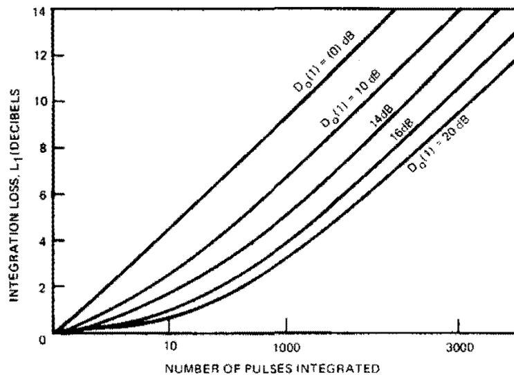
**Figure 13. Integration Loss Versus Number of Pulses Integrated for Different Values of Single-Pulse SNR**
