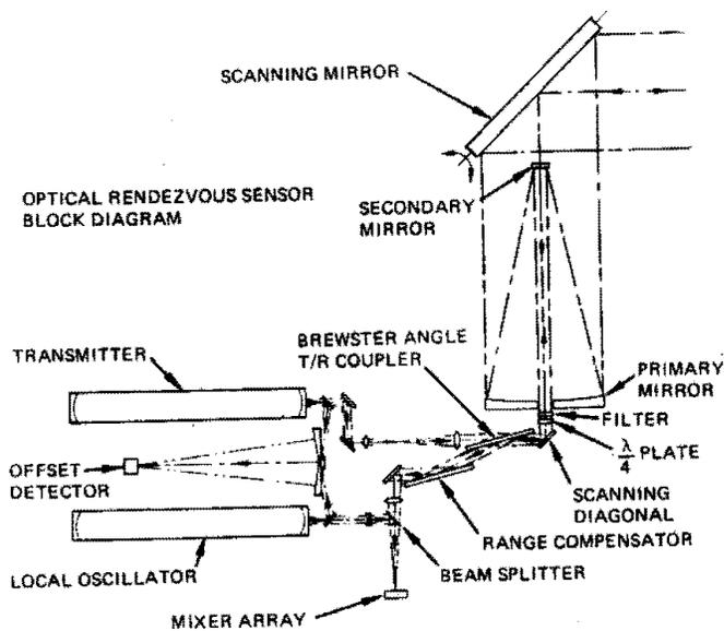
Figure 6. Optical Schematic of CW Laser Radar
