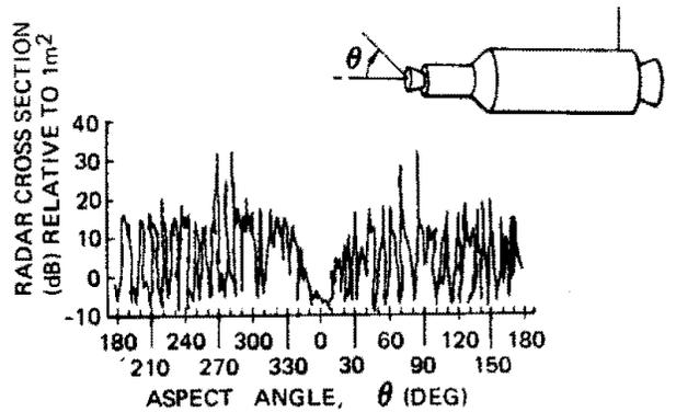
Figure 7. Measured Radar Cross Section of Agena Spacecraft at X Band
