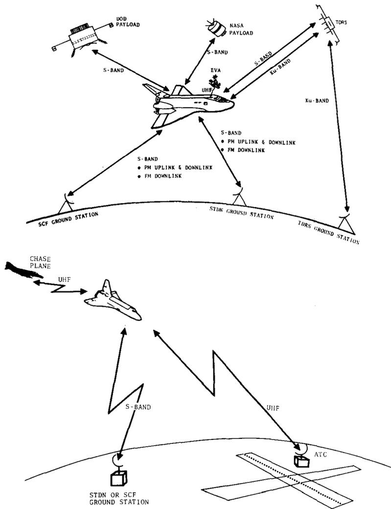
**Figure 3.- Shuttle communications**
