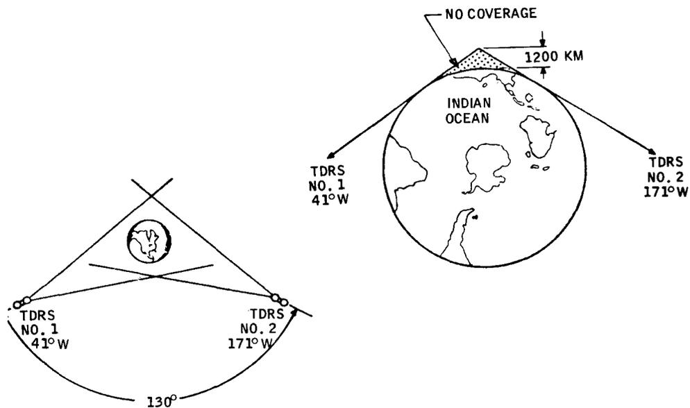
Figure 4.- Tracking and Data Relay Satellite System
