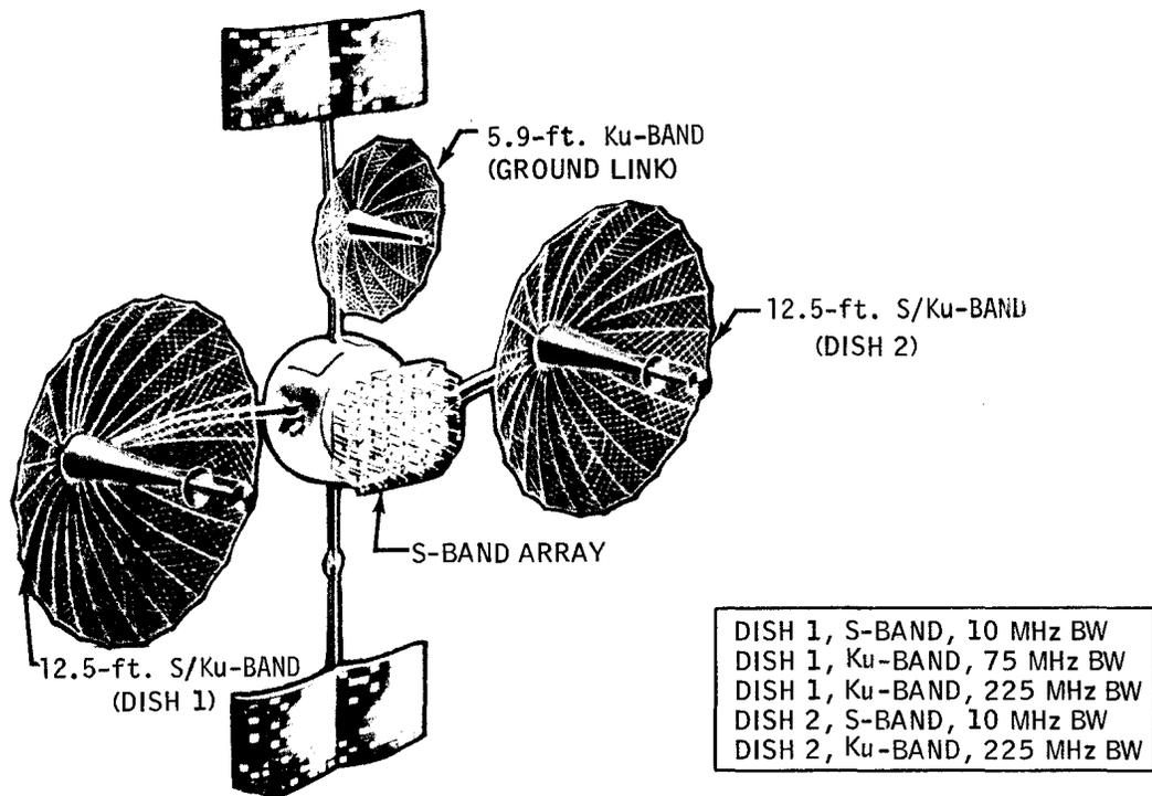
NOTE: S-BAND ARRAY IS FOR LOW DATA RATE USERS AND CAN HANDLE UP TO 20 SIMULTANEOUSLY. IT IS NOT UTILIZED BY SHUTTLE.
