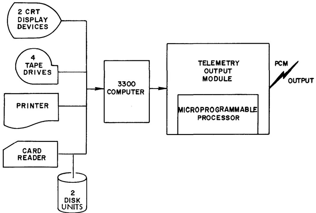
**FIGURE 1. TDVS HARDWARE CONFIGURATION**
