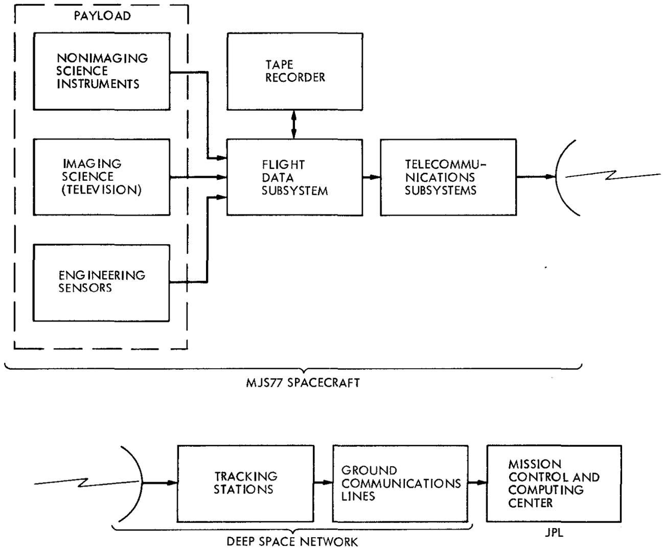
**Fig. 1. MJS77 telemetry system block diagram**
