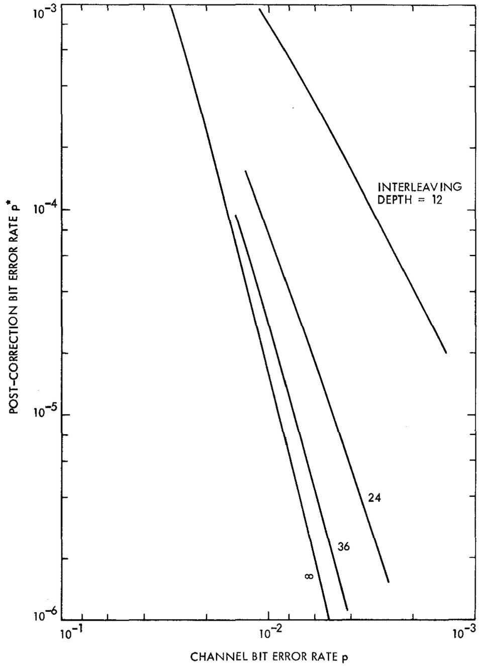
**Fig. 2. Error correction performance of MJS77 concatenated coding**
