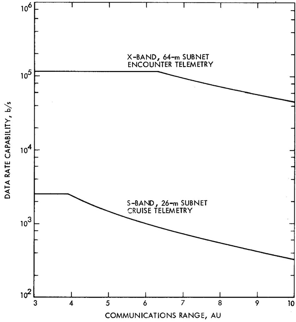
**Fig. 3. Nominal data rate capability of the MSS77 telemetry system**
