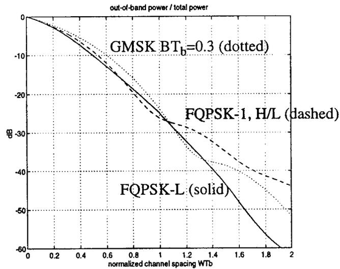
**Fig.4** Out-of-Band Power vs. Normalized Channel Spacing plot for FQPSK-L, FQPSK- I with hardlimiter and GMSK  $BT_b=0.3$ .
