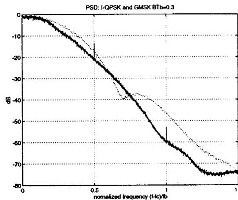
**Fig.3** Power Spectrum Density of FQPSK-L (solid) and GMSK  $BT_b=0.3$  (dotted)
