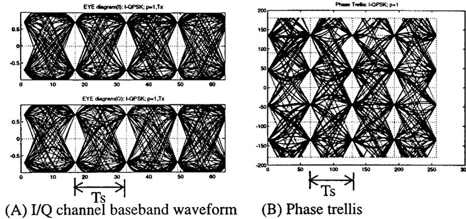
**Fig.2** I/Q channel baseband waveforms and phase trellis of FQPSK-L
