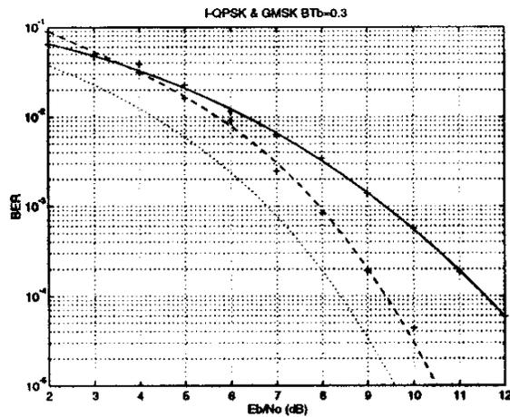
**Fig.5** BER performance of coherent FQPSK-L (solid), GMSK BTb=0.3 (dashed), and ideal QPSK dotted .
