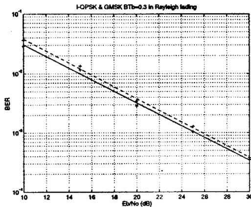
**Fig.7** BER performance of FQPSK-L and GMSK BTb=0.3 as function of  $E_b/N_0$  in Rayleigh fading channel. FQPSK-L outperforms GMSK by 0.8 dB.
