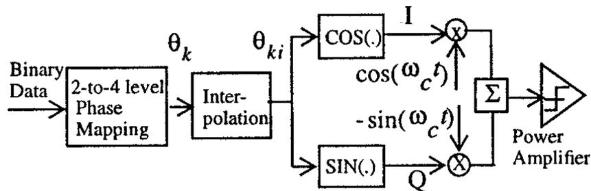
**Fig.1** Block diagram of the transmitter of FQPSK-L system.
