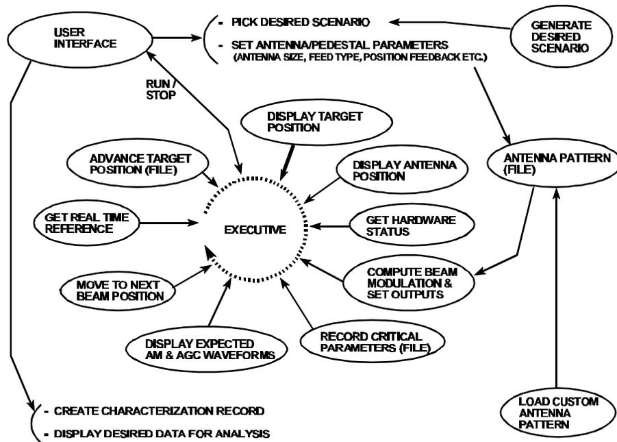
Figure 3 - Functional Description of Telemetry Environment Simulator (TES) Operation
