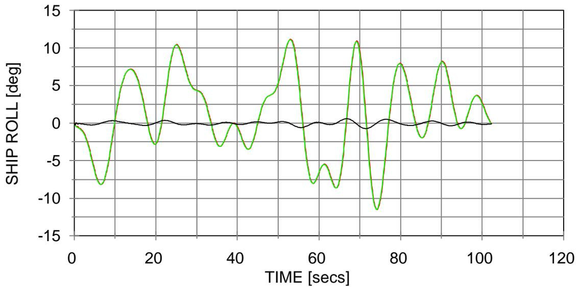
Figure 7 - Pedestal Response Quantifiably Improved With Modified Tracking Algorithm
