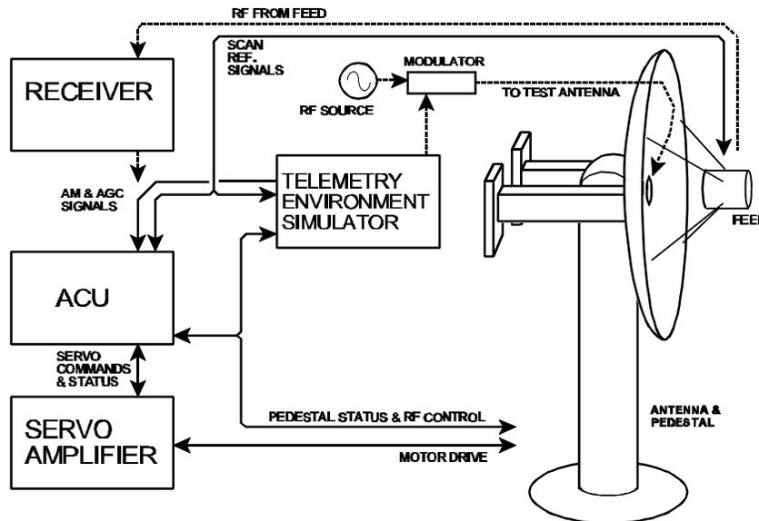
**Figure 1 - Typical Application of Telemetry Environment Simulator (TES). Dotted Lines Show RF Signal Injection Path.**
