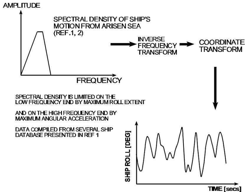
**Figure 5 - Pictorial Description of AM Waveform Generation**
