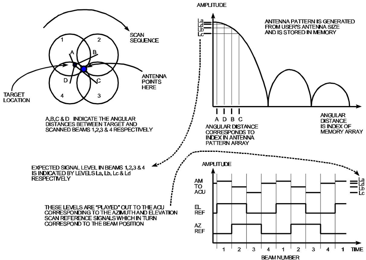
**Figure 4 - Pictorial Description of AM Generation in the TES**
