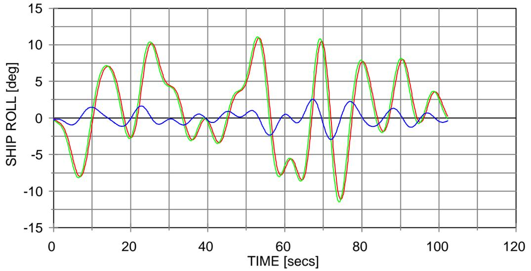
Figure 6 - Pedestal Response in Simulated "Sea State 5" Conditions
