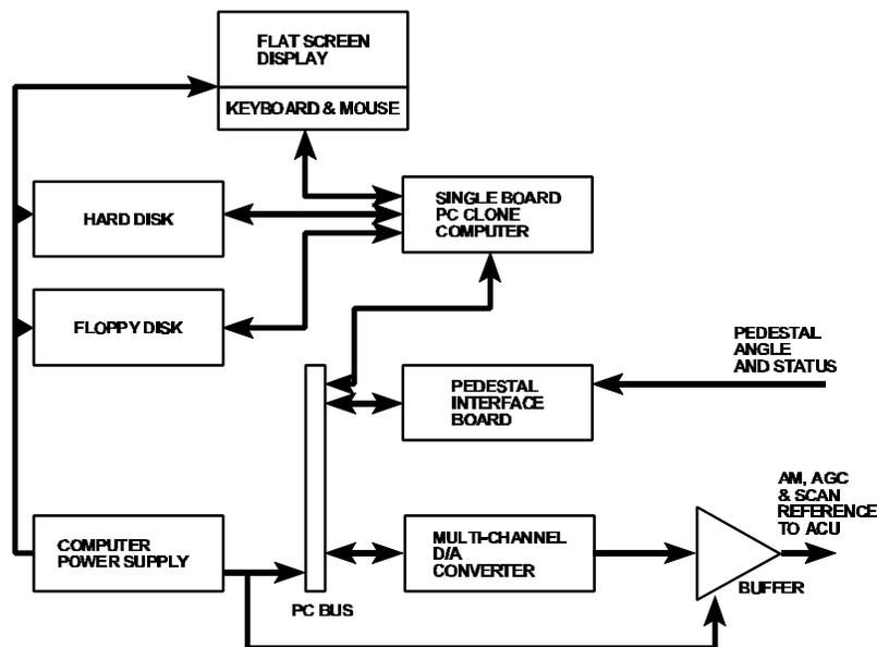
Figure 2 - Functional Block Diagram of TES Hardware
