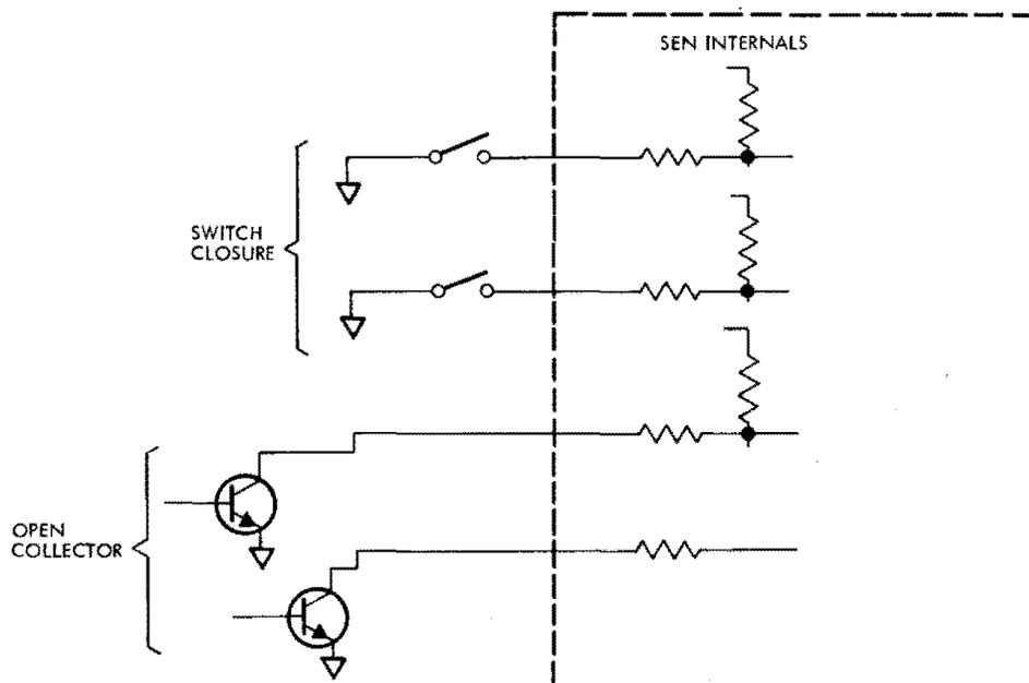
**Fig. 9 - SEN Input Circuit Configurations.**
