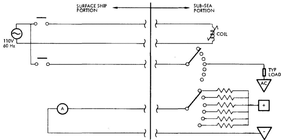
**Fig. 1 - Stepper Switch Command System.**
