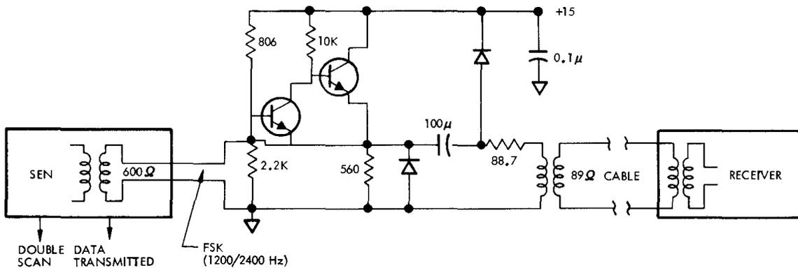
**Fig. 8 - Cable Driver Receiver.**
