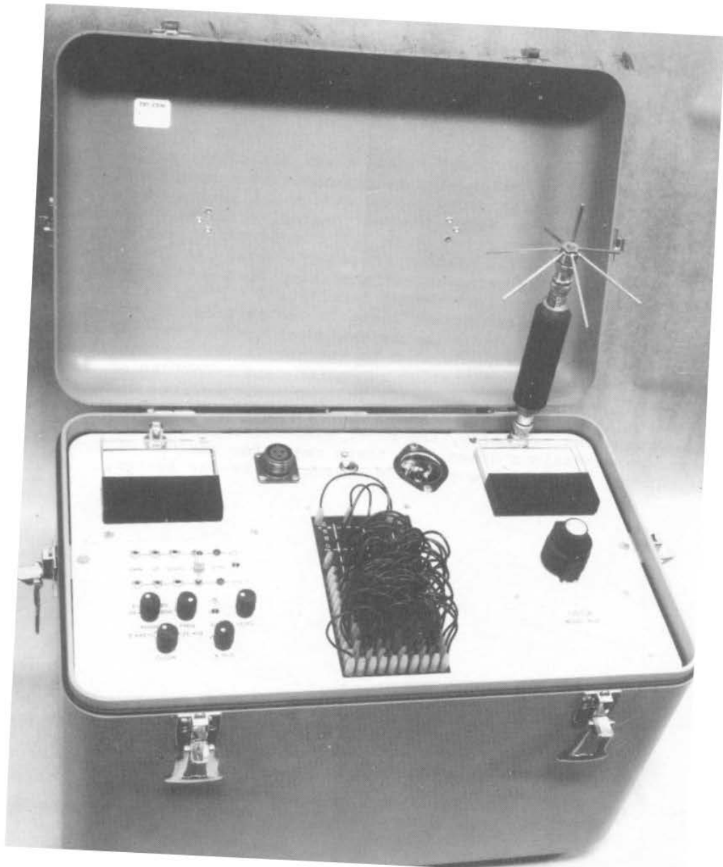
FIGURE #10 RF TEST BOX - MISSILE TLM DYNAMIC TEST SET - CAN SIMULATE MISSILE TLM FROM BIRD IN FLIGHT
