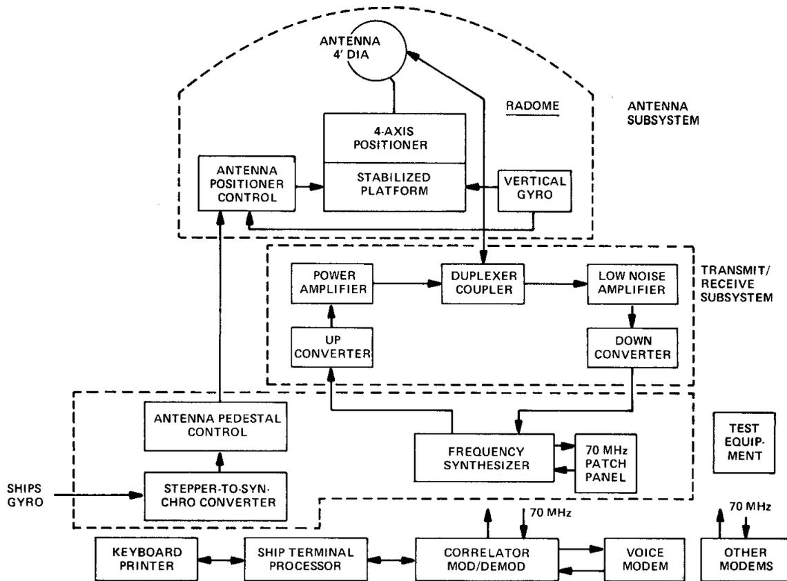
**Fig. 4 - Simplified Diagram of Ship Communications Terminal**
