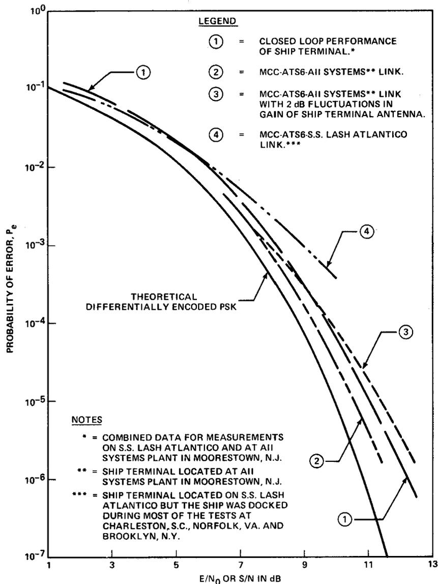
**Fig. 10 - Ship Terminal Performance of Magnavox Modem at 9600 BPS.**
