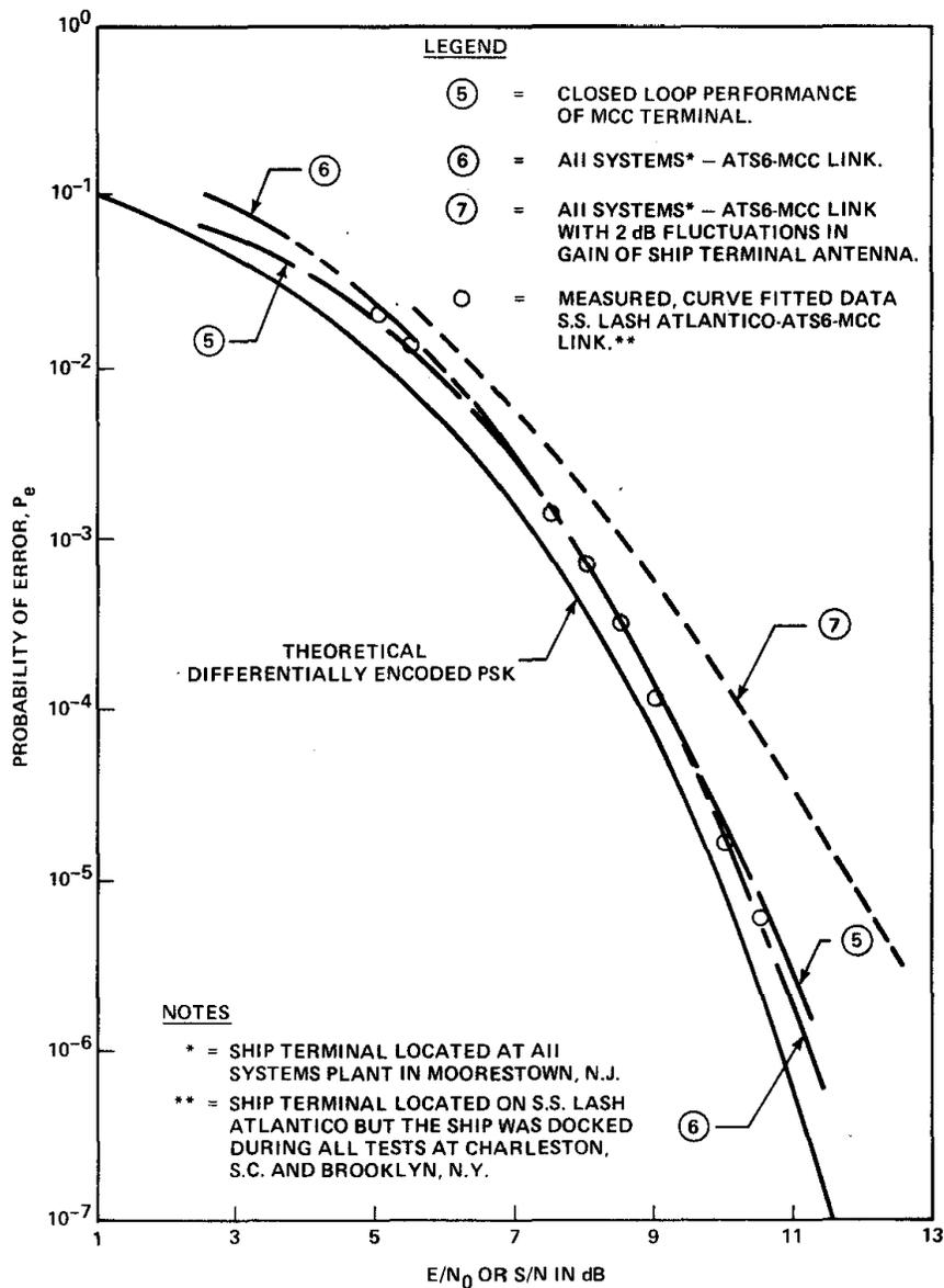
**Fig. 11 - Maritime Coordination Center (MCC) Performance of Magnavox Modem at 9600 BPS.**
