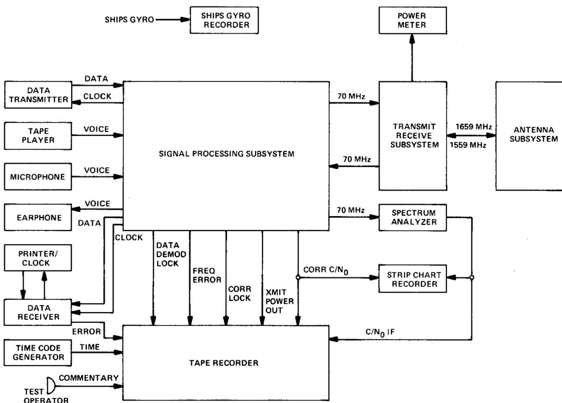
**Fig. 9 - LASH Atlantico Shipboard Instrumentation for Data Tests.**
