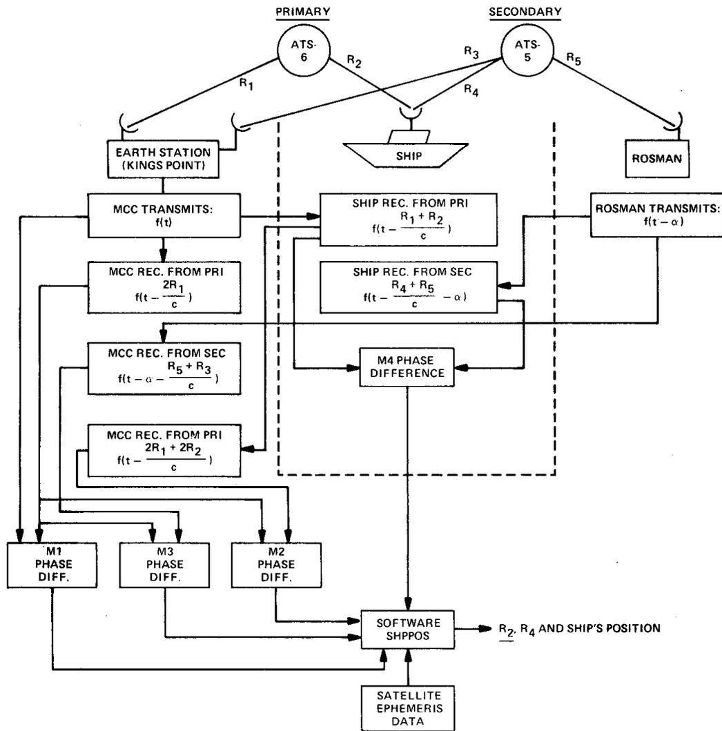
**Fig. 7 - Position Determination Block Diagram.**
