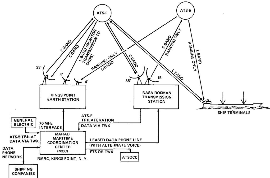
**Fig. 1 - MARAD L-Band Experimental Configuration**
