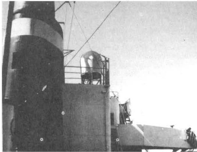
**Fig. 2 - Ship Antenna Terminal on the American Ace.**
