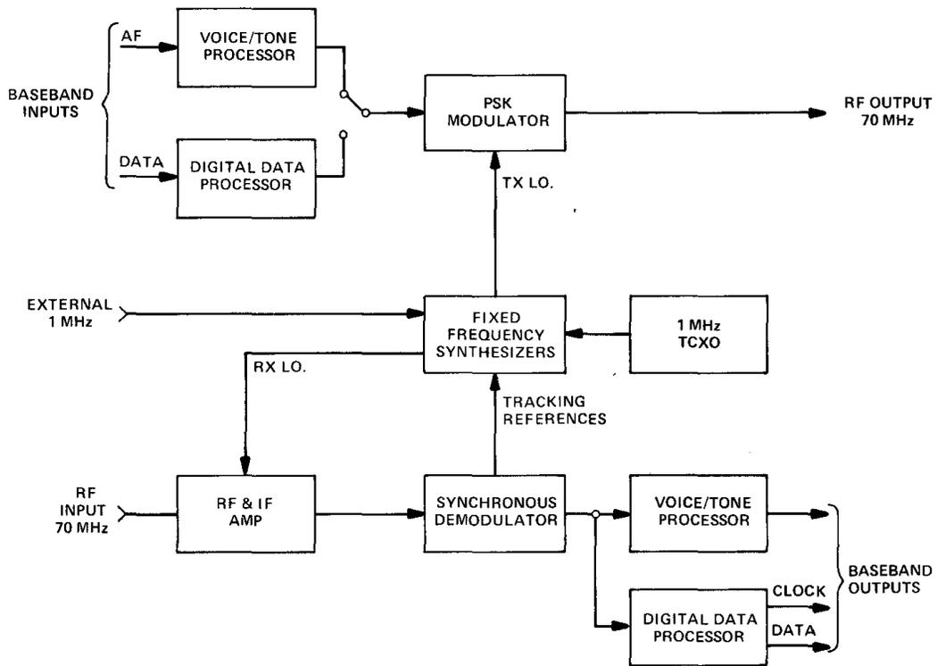
**Fig. 5 - Simplified Magnavox Modem Block Diagram.**
