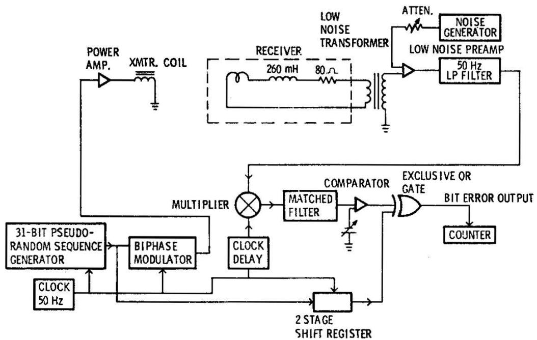
**FIGURE 4. Block Diagram of Simulated Telemetry System**
