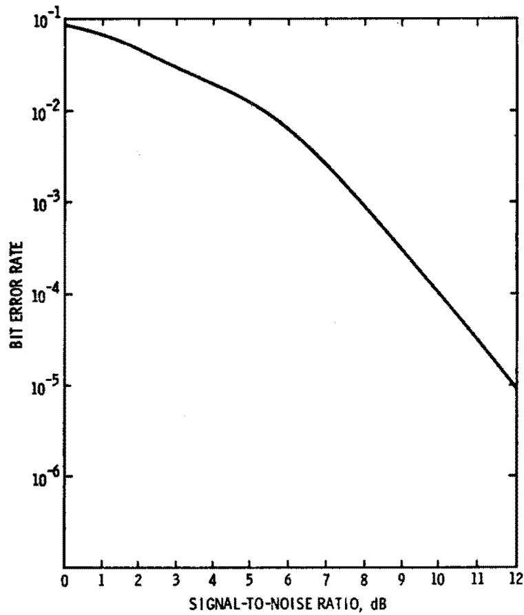
**FIGURE 5. Bit Error Rate versus Signal-to-Noise Ratio for Simulated Telemetry System**
