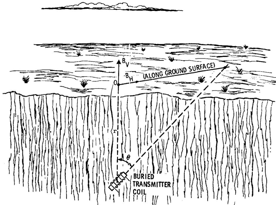
**FIGURE 1. Geometric Variables involved in Underground-to-Surface Telemetry Link**
