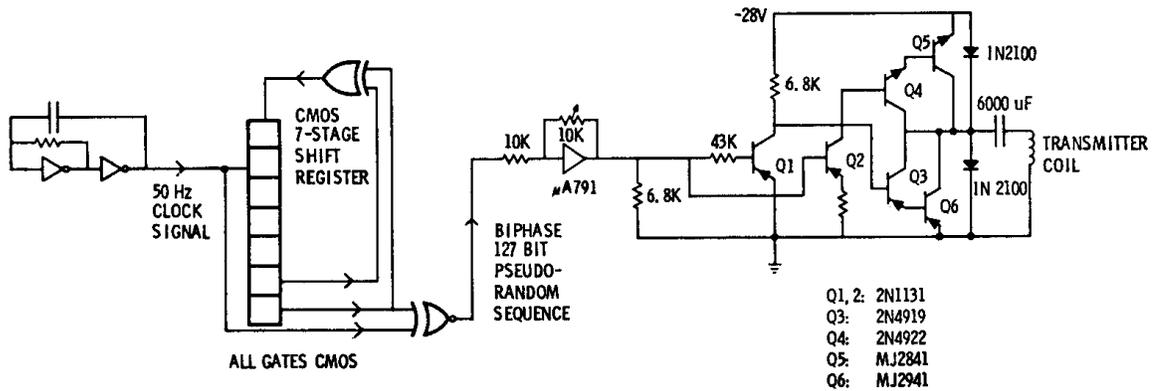
**FIGURE 6. Transmitter Driver Schematic**
