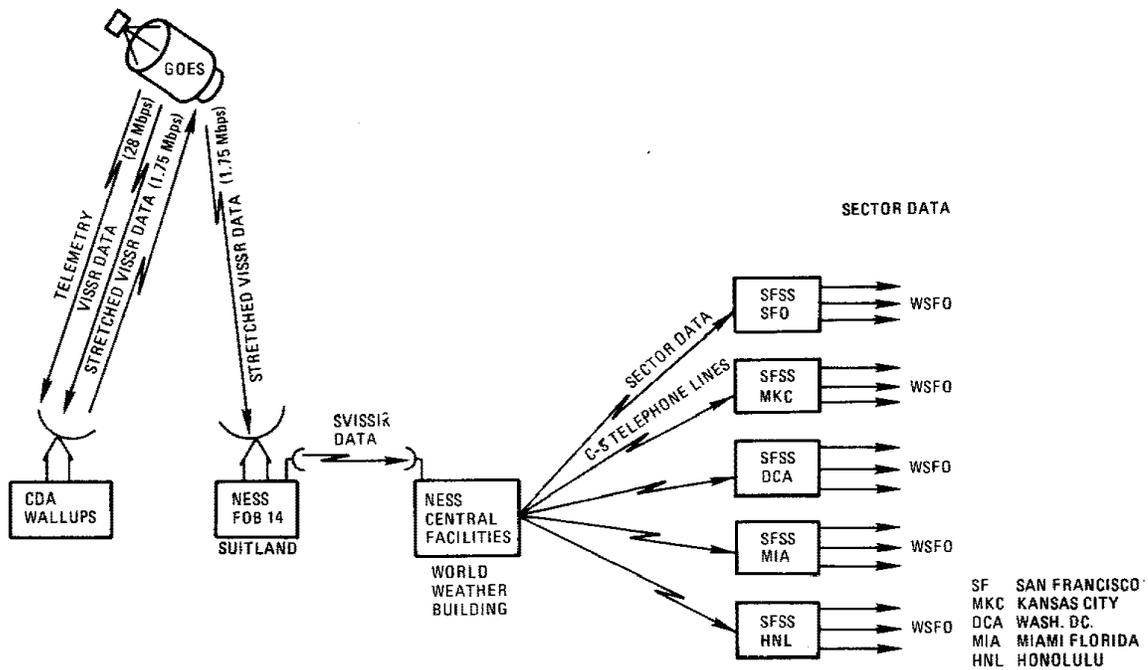
**Figure 2 The GOES Imaging Communications System**
