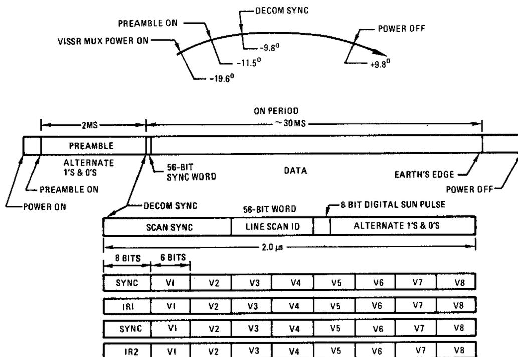
**Figure 6 Data Format for VISSR Transmission**
