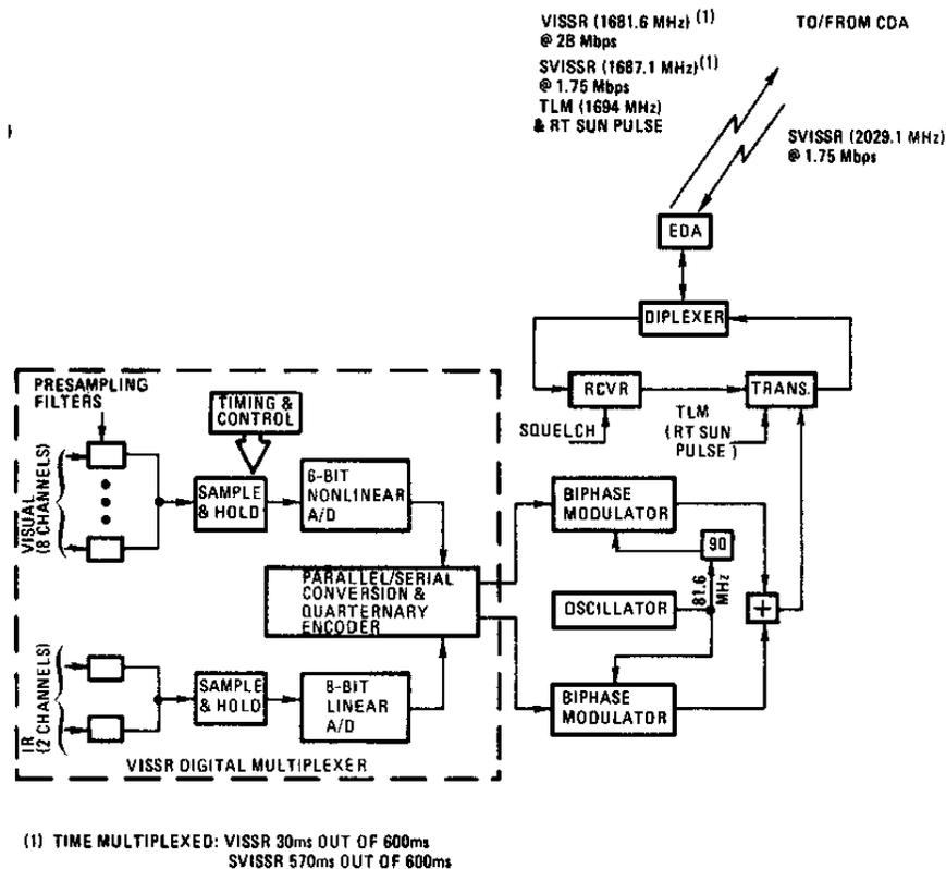
**Figure 5 Simplified Functional Block Diagram of the GOES Segment**
