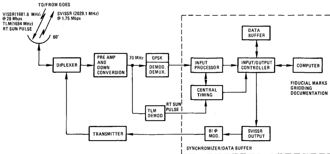
**Figure 7 Simplified Block Diagram of CDA Segment**
