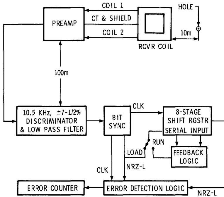
**Figure 6. Diagram of Receiving System**
