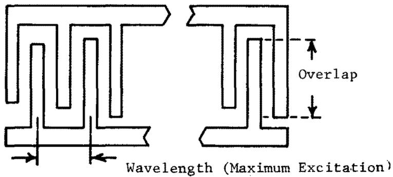
**FIGURE 2. INTERDIGITAL TRANSDUCER**
