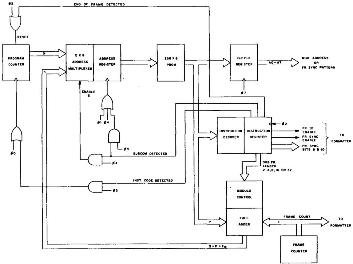
Fig. 7 PR-614 Processor Block Diagram
