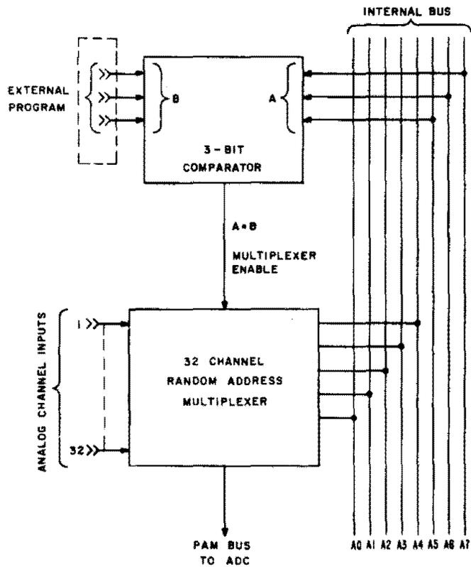
**Fig. 5 MP-601 Analog Multiplexer Block Diagram**
