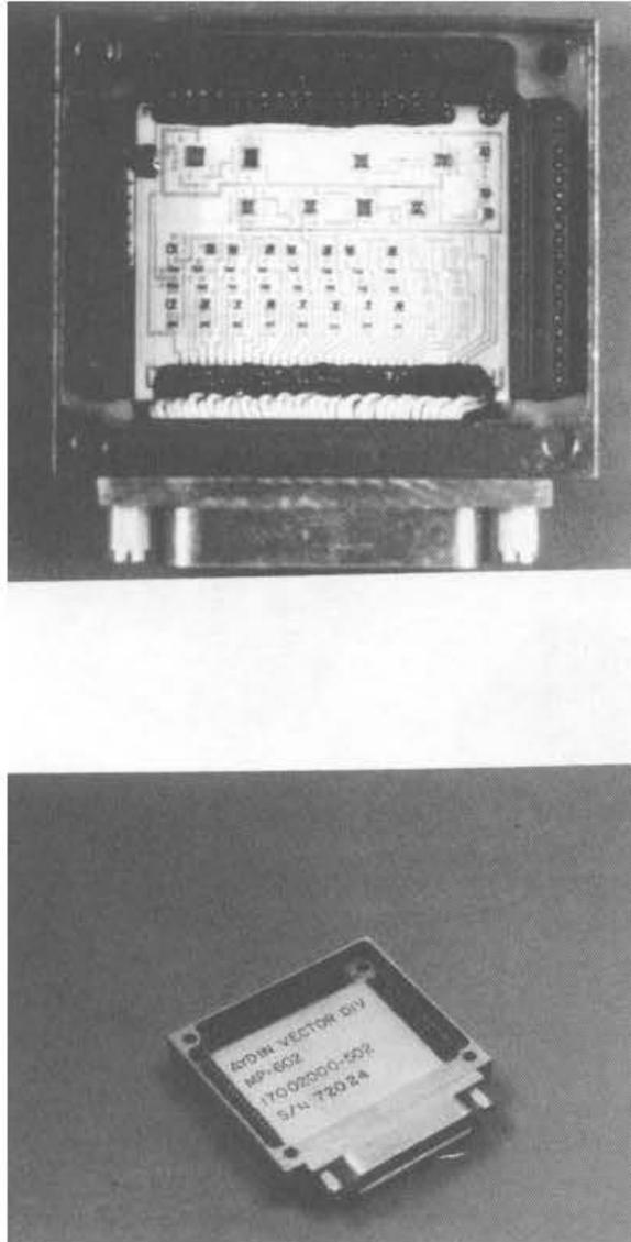
**Fig. 2 Typical PCM Module with Cover Off and On**
