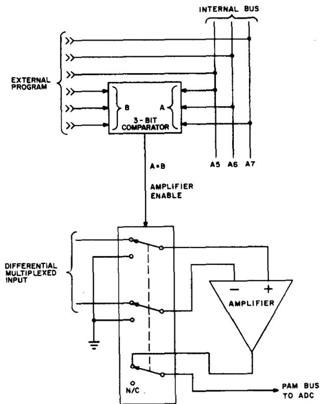
**Fig. 6 Differential Amplifier Functional Diagram**
