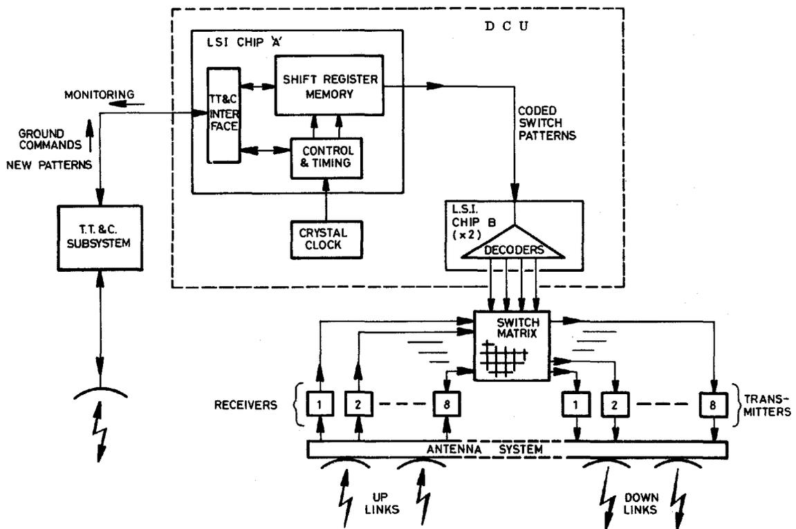
FIG. 3 MAJOR DCU FUNCTIONS WITHIN SATELLITE SYSTEM
