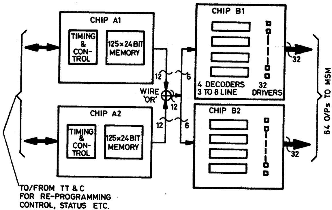
FIG. 4 PARTITION INTO FOUR CHIPS
