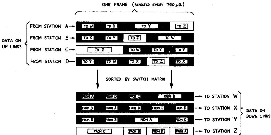
FIG. 2 PART OF EXAMPLE CONNECTION PATTERN
