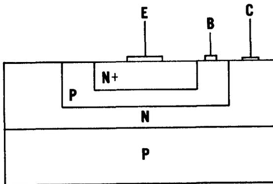
Figure 1. A Bipolar Transistor
