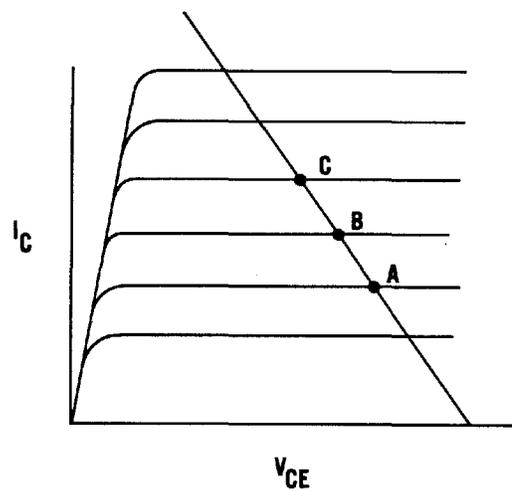
Figure 6.  $V_{CE}$ - $I_C$  Characteristic
