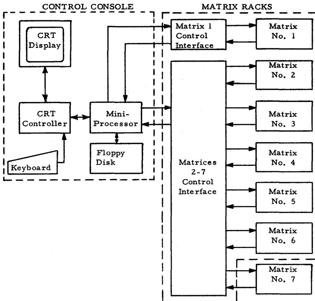
**Figure 1. ADESS Functional Block Diagram**
