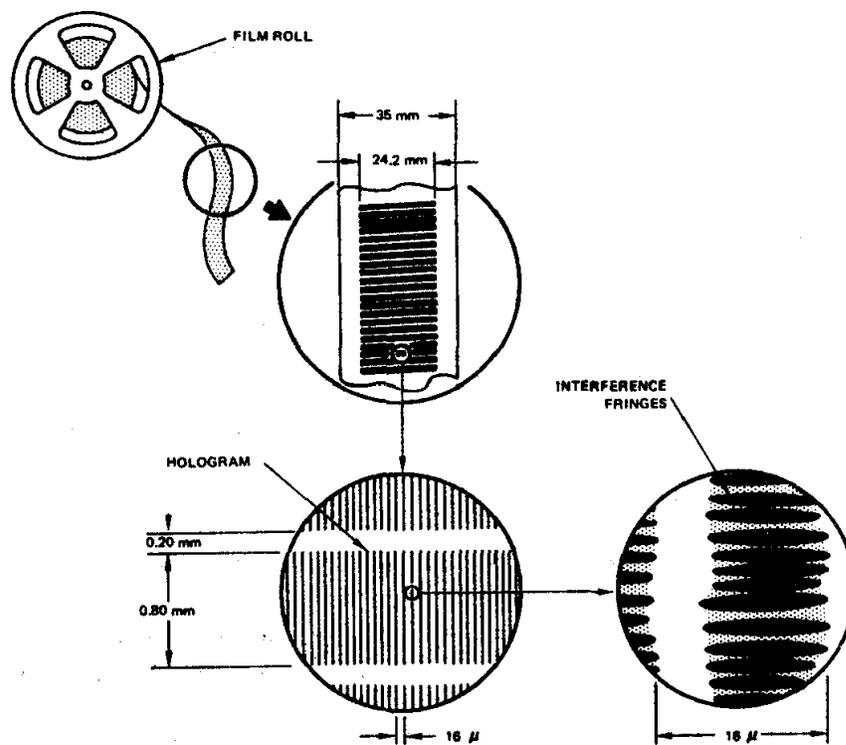
**Fig. 7 - Wideband Recorder Film Format**
