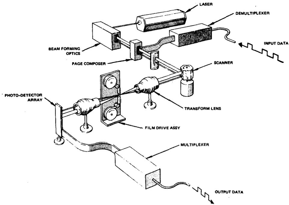
**Fig. 8 - Wideband Holographic Recorder**
