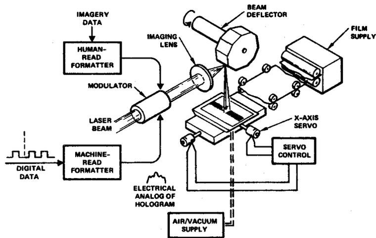
**Fig. 4 - Record Conceptual Diagram**
