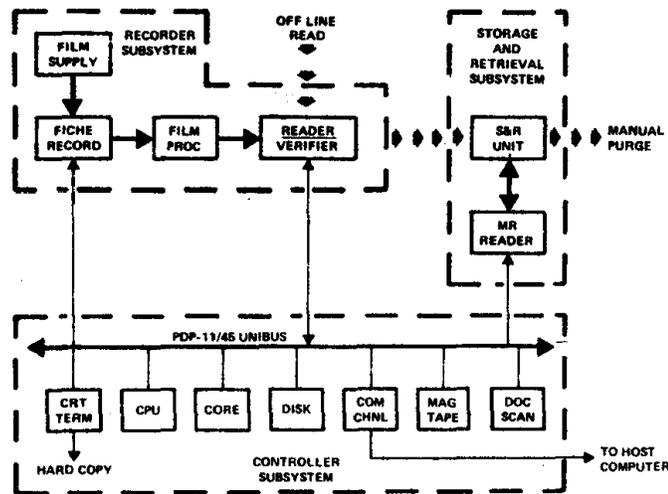
**Fig. 2 - HRMR System Block Diagram**
