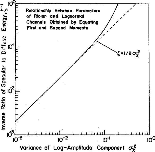
Figure 2 Relationship Between Parameters of Rician and Lognormal Channel
