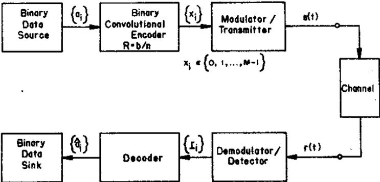
Figure 1 MFSK System Employing Binary Convolutional Coding
