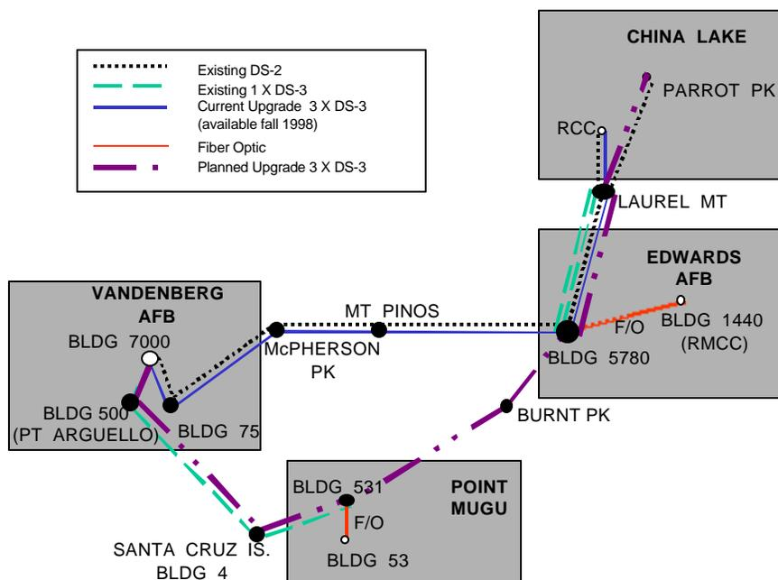
**Figure 1. Inter-Range Microwave Communications Architecture.**
