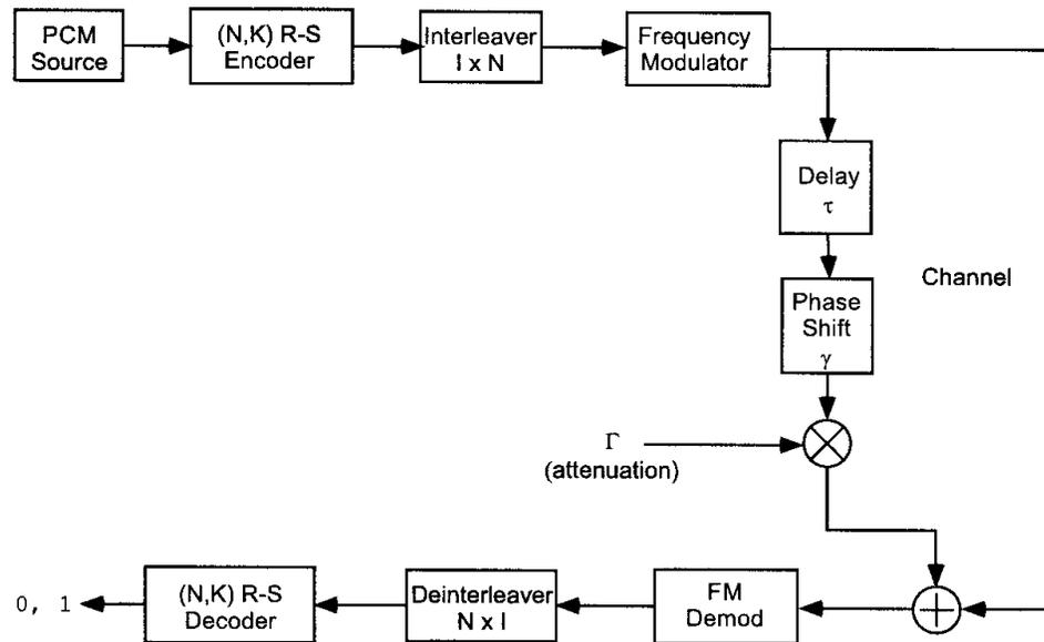
Figure 4: Block Diagram of PCM/FM Aeronautical Communication System
