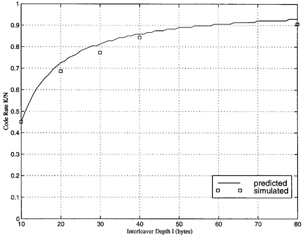
Figure 5: Simulated vs Predicted Code Rates for Sweep Rate of 27 GHz/sec
