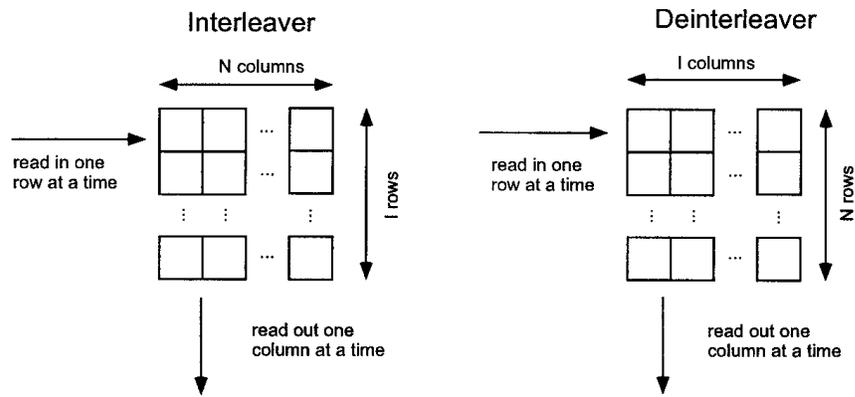
Figure 1:  $I \times N$  Block Interleaver
