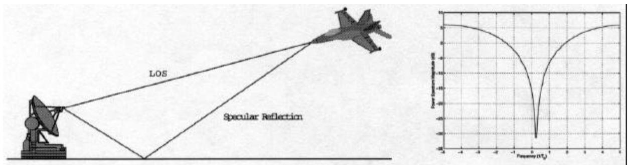
Figure 2: Multipath Channel Configuration and Plot of  $|H(f)|^2$  for  $\gamma = \gamma_0 - .05\pi$
