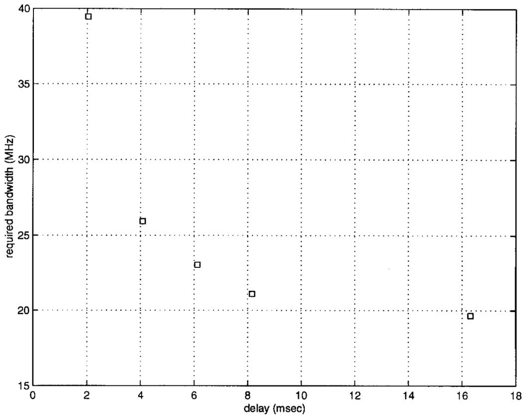
Figure 3: Bandwidth Expansion vs Interleaving Delay for Sweep Rate of 27 GHz/sec
