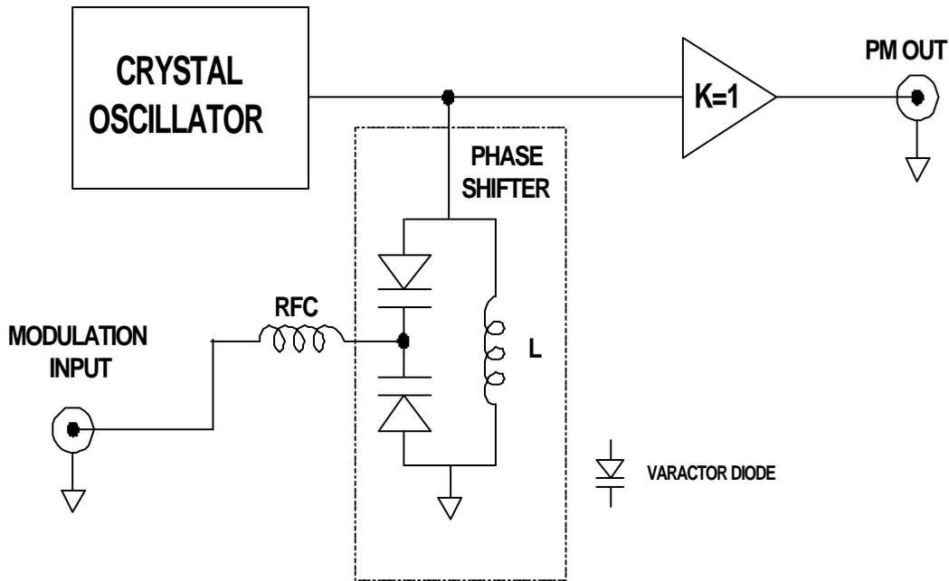
**Figure 1 Full Deviation RF Phase Modulator**
