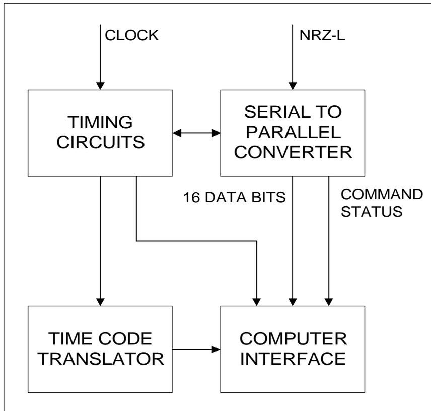
**Figure 5. Block Diagram of Decoding Circuit**
