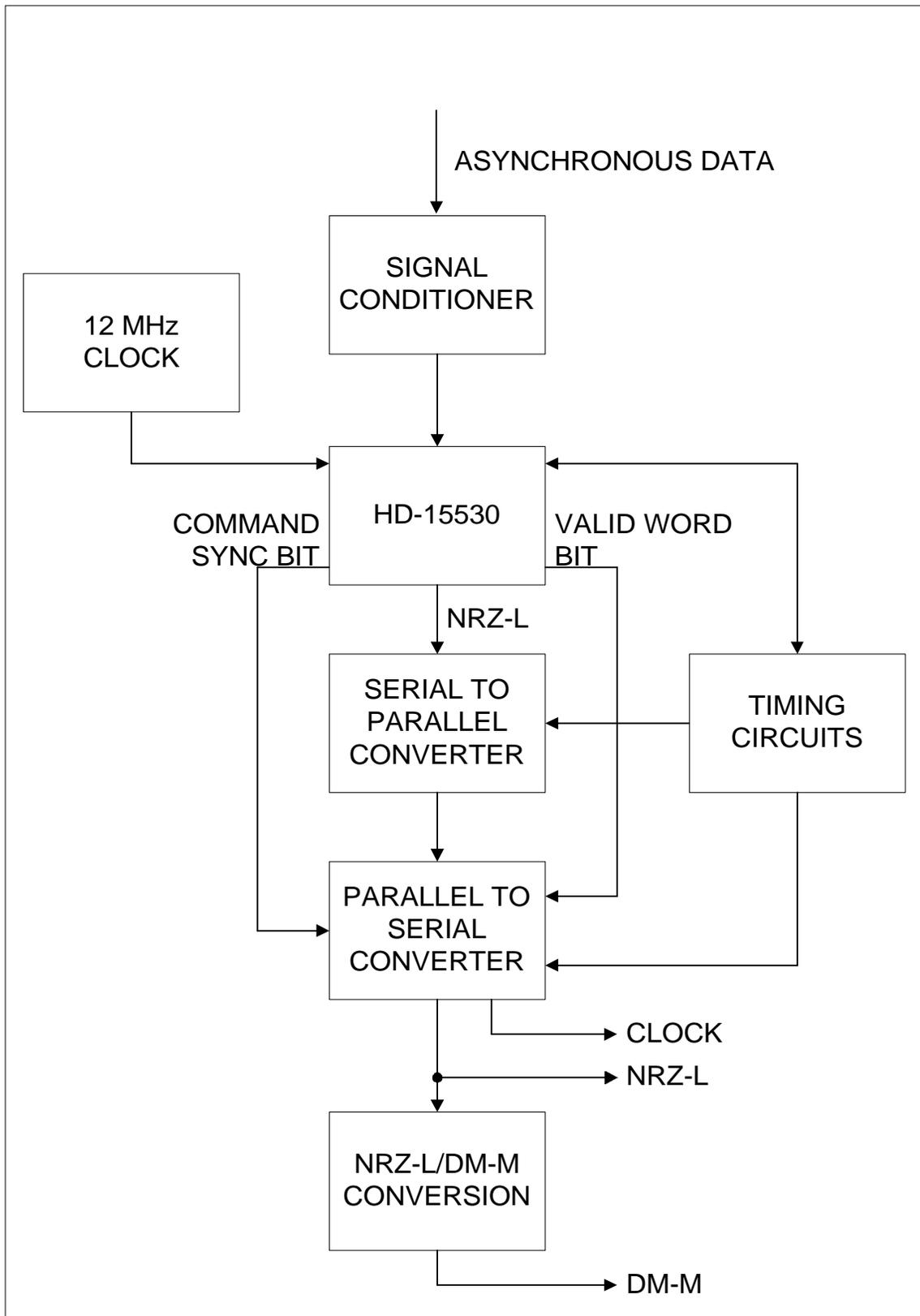
**Figure 2. Block Diagram of Encoding Circuit**
