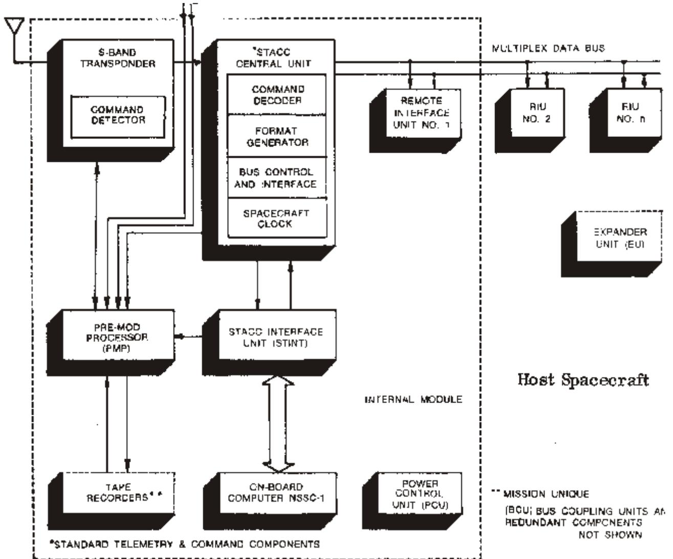
**Figure 1. SIMPLIFIED C&DH SUBSYSTEM BLOCK DIAGRAM**
