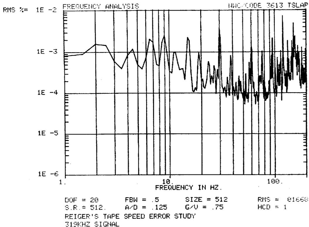
**Figure Three: Tape Flutter Plot--Recorder and Playback Machines Combined**
