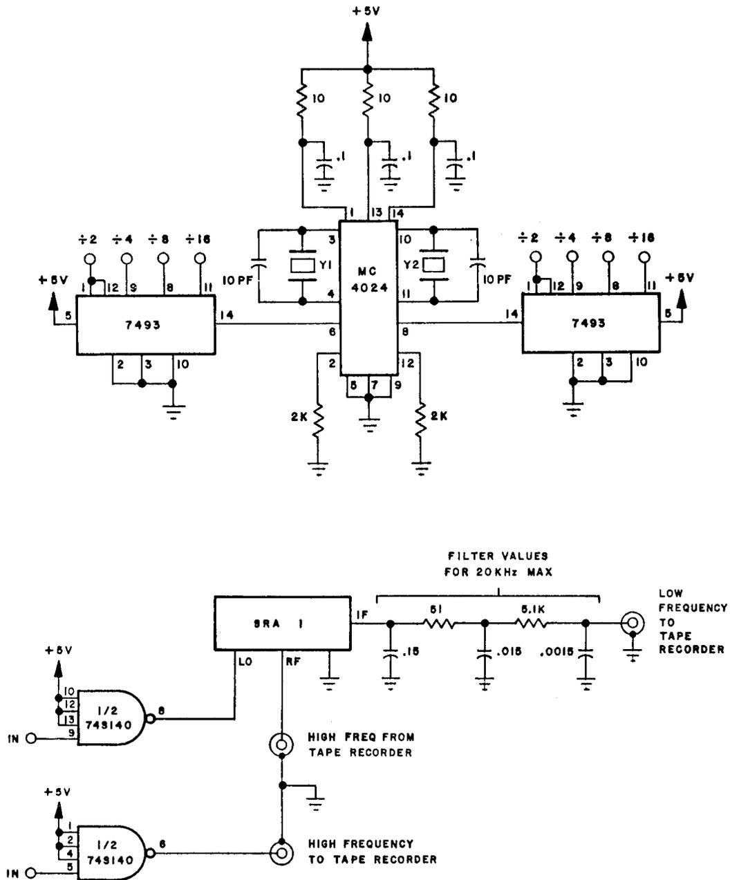
Figure One: Circuits Used in Flutter Signal Translator
