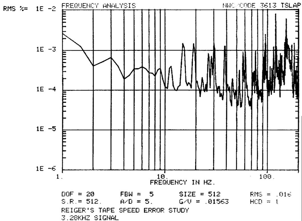
**Figure Two: Tape Flutter Plot--Recorder Only**
