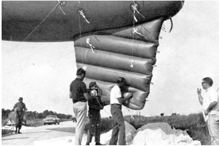
**Fig. 4 - Measuring Balloon's Internal Pressure**
