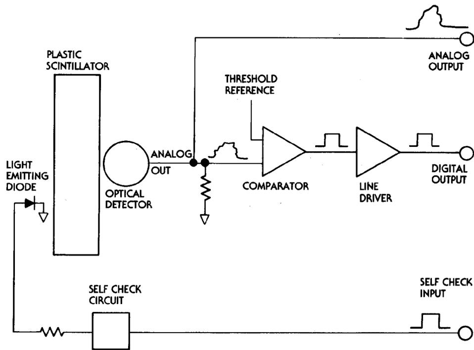
**Figure 2. Diagram of Neutron Detector**
