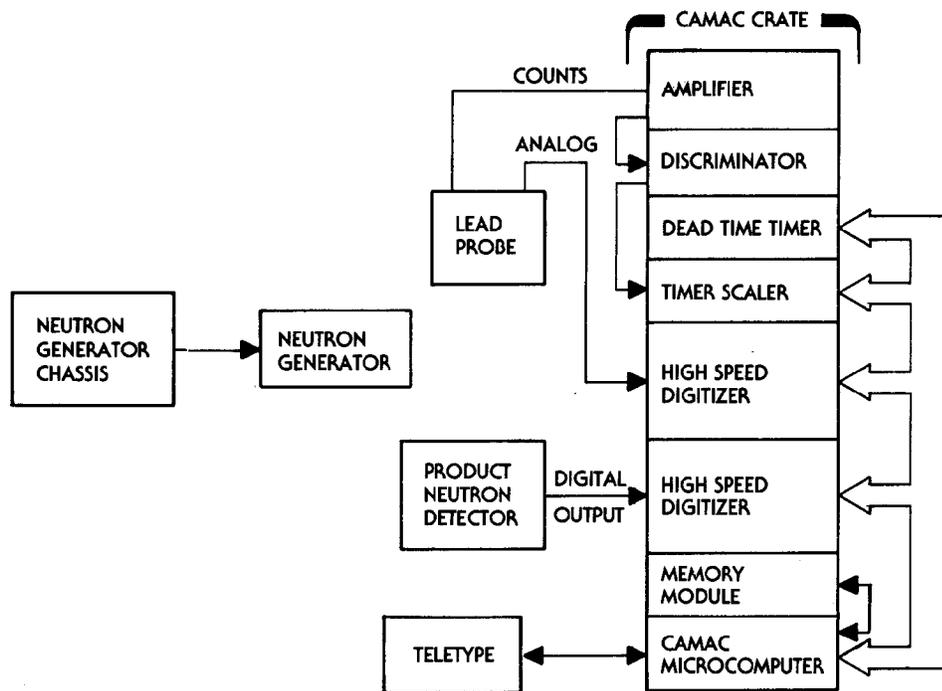
**Figure 5. Block Diagram of Test System**
