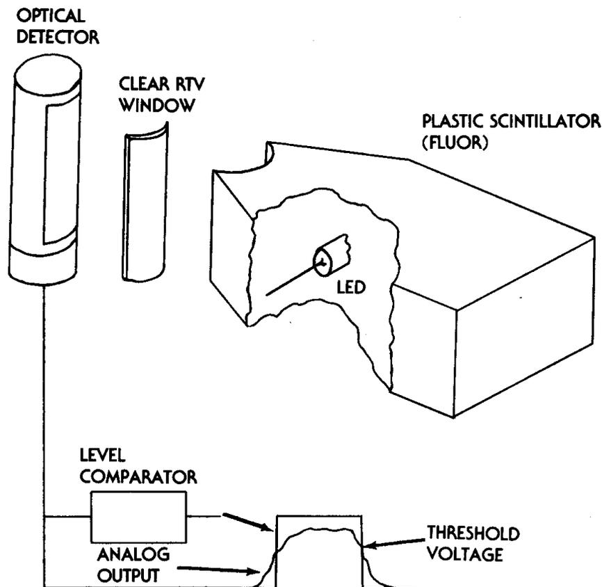
**Figure 1. Miniature Neutron Detector**
