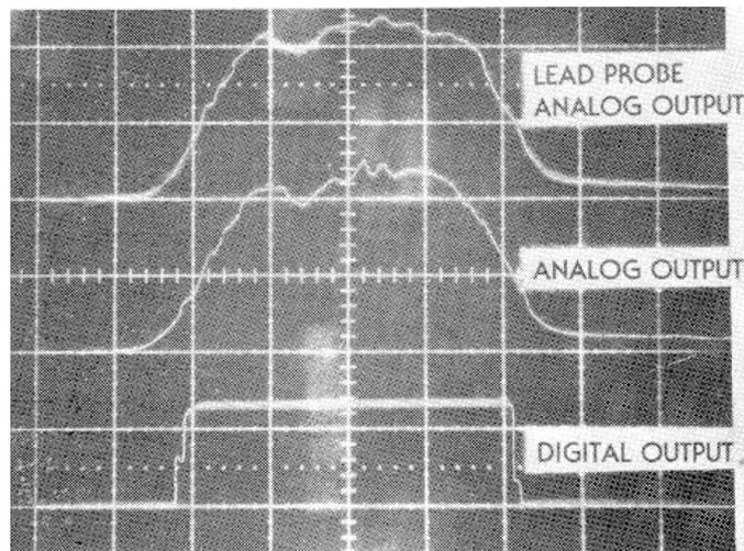
**Figure 3. Oscilloscope Display of Output From Neutron Detectors**
