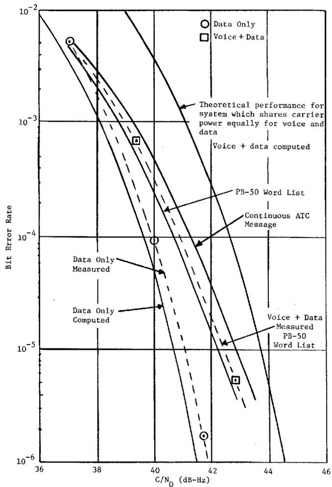
**Figure 8. Hybrid Modem 1200 bps Data Error Rate Performance**
