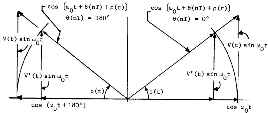
Figure 4. Voice and Data Quadrature Modulator Vector Diagram
