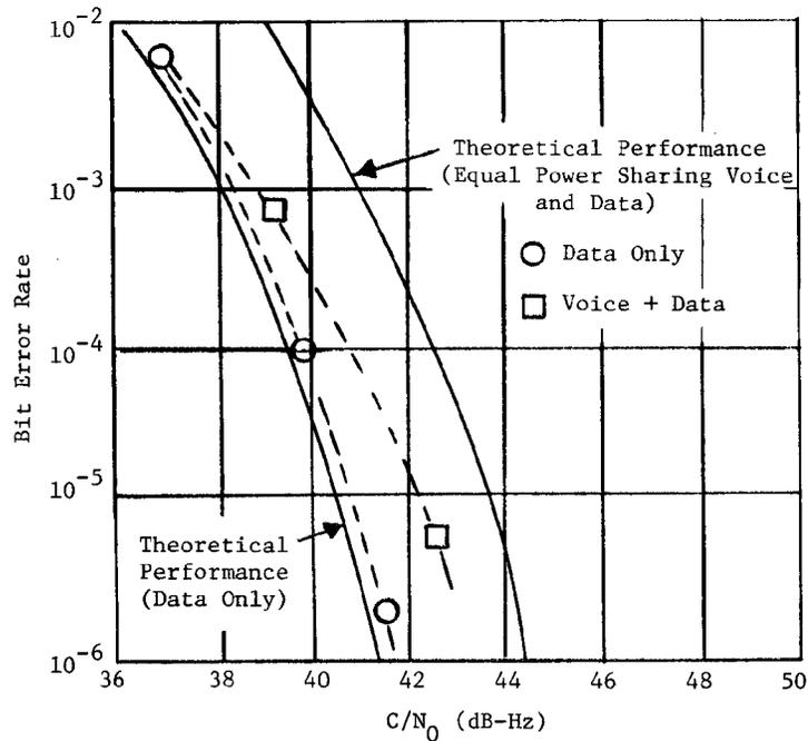
Figure 6. Hybrid Modem 1200 bps Data Error Rate Performance
