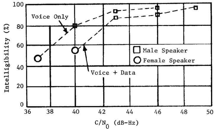
Figure 5. Hybrid Modem Voice Intelligibility Test Results
