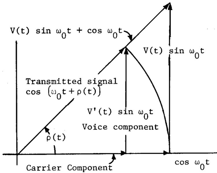
Figure 2. Quadrature Modulator Vector Diagram
