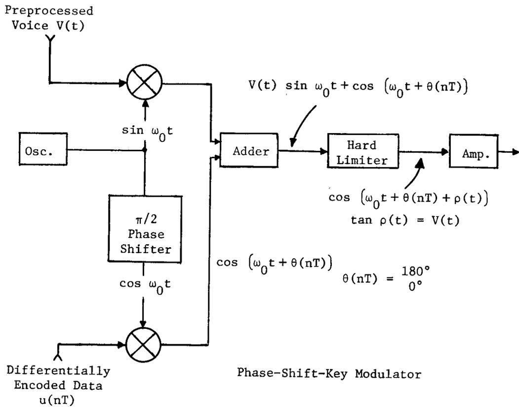
Figure 3. Voice and Data Quadrature Modulator
