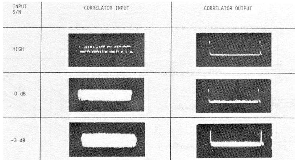
**Figure 8. Matched Filter Correlator Inputs/Outputs**
