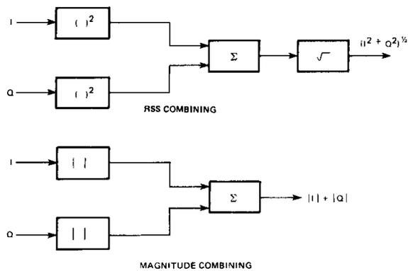
Figure 10. Noncoherent Combining
