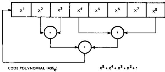
**Figure 16. 8 Stage 255 Element LSRG**
