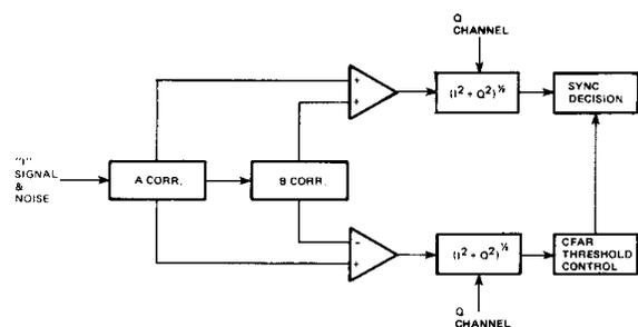
Figure 12. Orthogonal CFAR implementation
