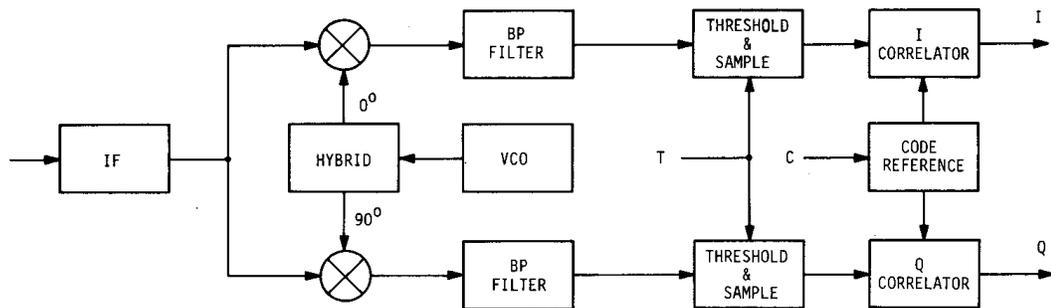
**Figure 9. Coherent Demodulator**
