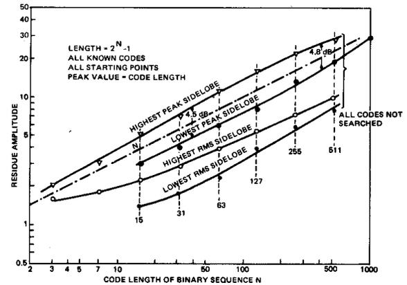
**Figure 5. Maximum and Minimum Values of Binary Phase-Coded Residues<sup>5</sup>**
