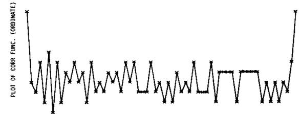
**Figure 3. Correlation Function of 63 Chip Pseudo-Random Sequence; with Alternate Chip Detection Errors**
