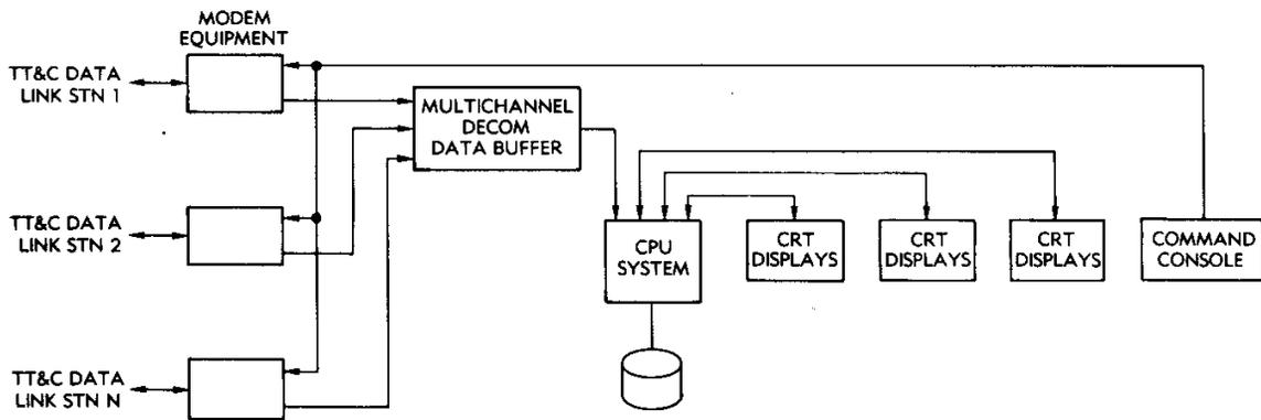
**Fig. 1 - A Centralized Control Center Configuration**
