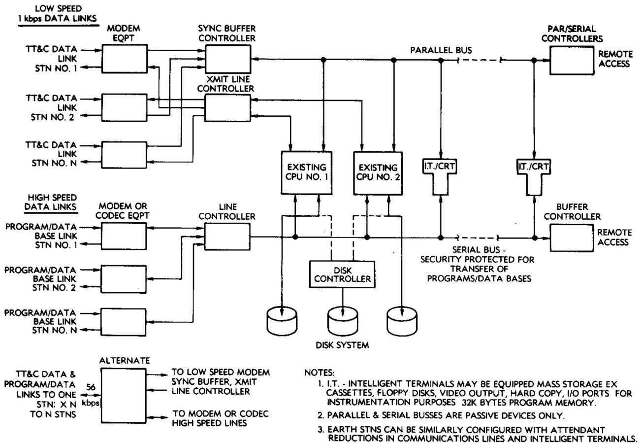
**Fig. 2 - Possible Future Control System for Automatic Commanding Using Distributed Processing Concepts**
