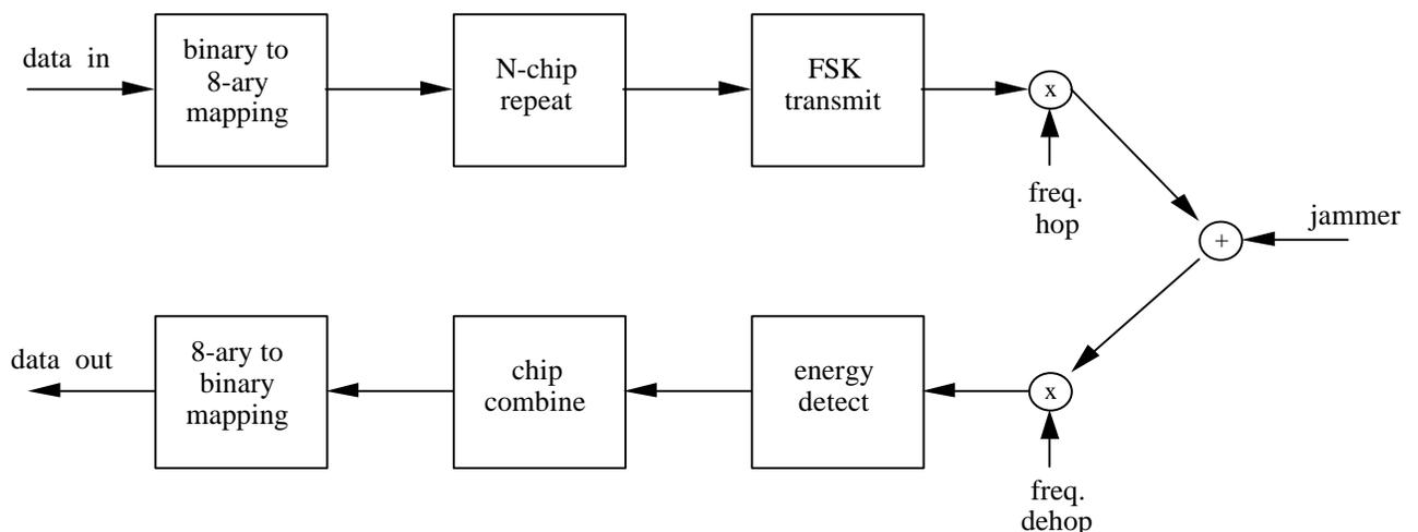
Figure 1: Fast Frequency Hopped System Model .
