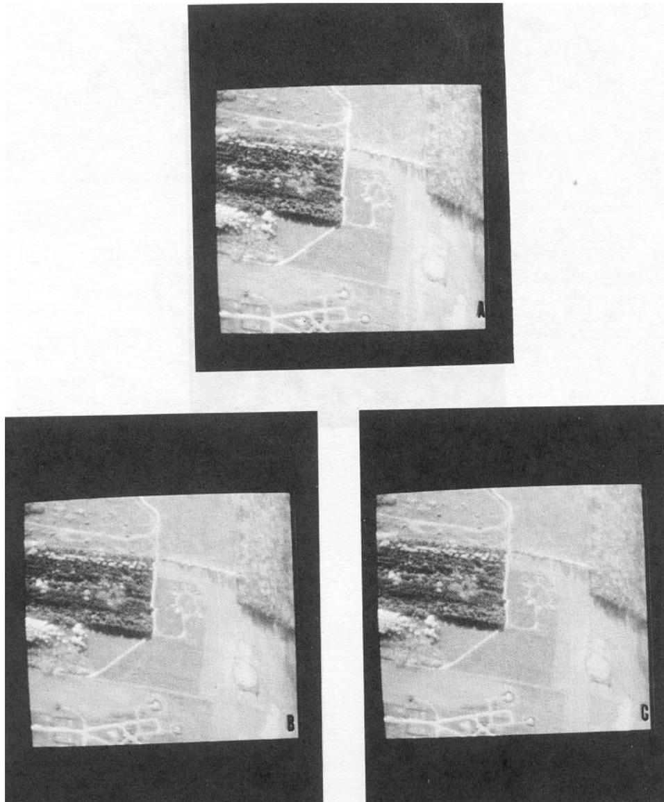
**Figure 5 Missile Site: a) 8 bit original, b) 2 bit adaptive DPCM, c) 2 bit non-adaptive DPCM**
