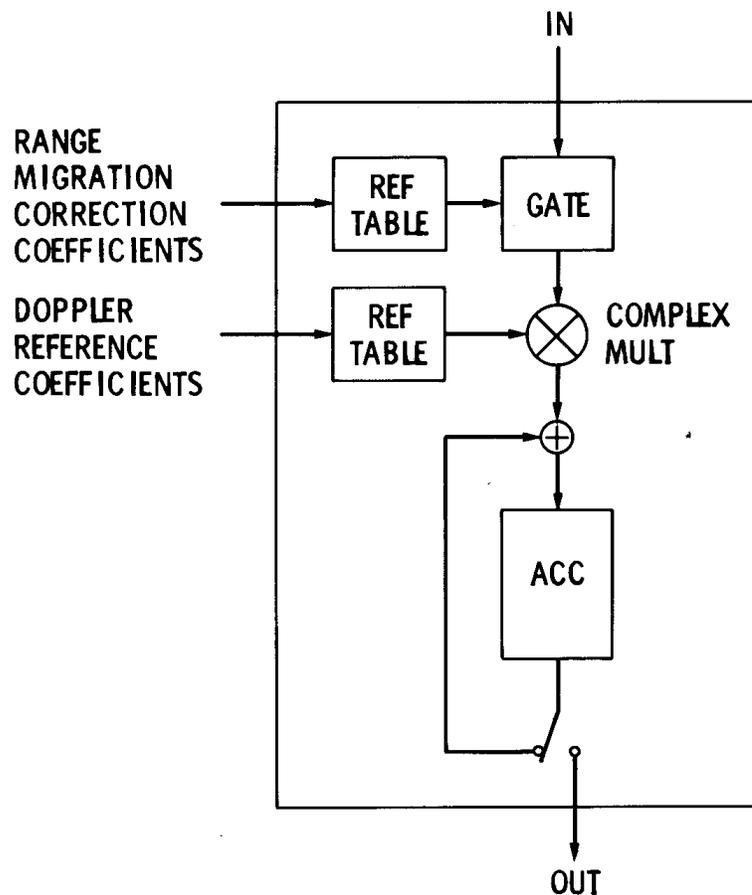
**Figure 5 - Azimuth Filter Chip.**
