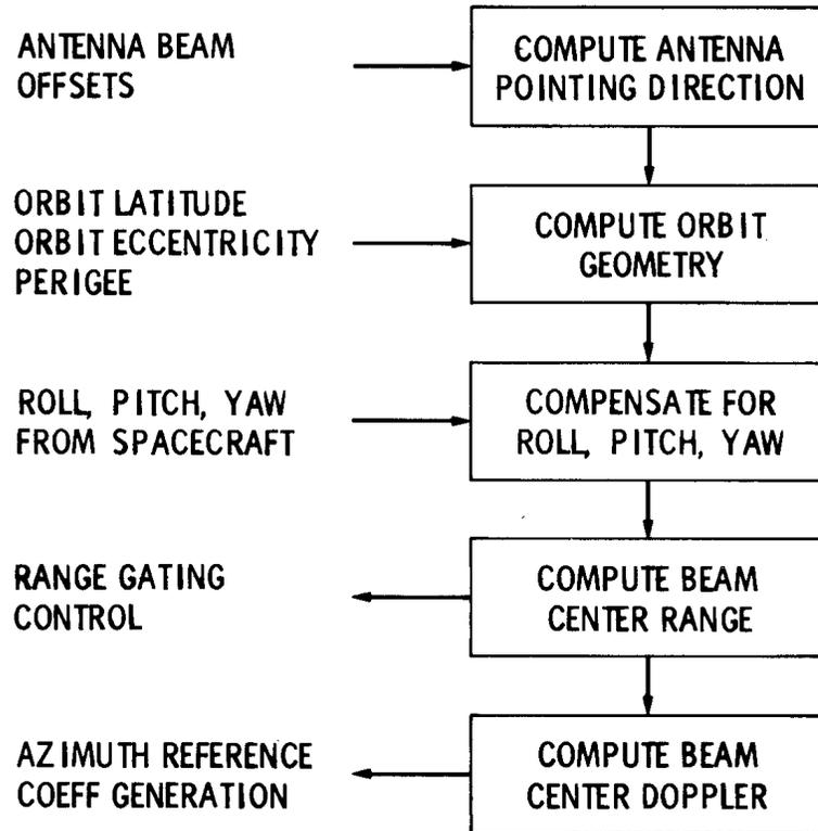
**Figure 7 - Beam Center Range and Doppler Offset Computations**
