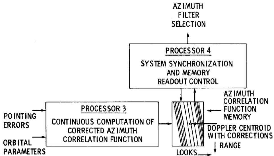
**Figure 9 - SAR Antenna Pointing Error Corrector Concept**
