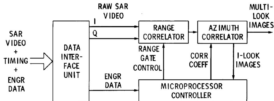
**Figure 1 - Real-Time SAR Processor Block Diagram**
