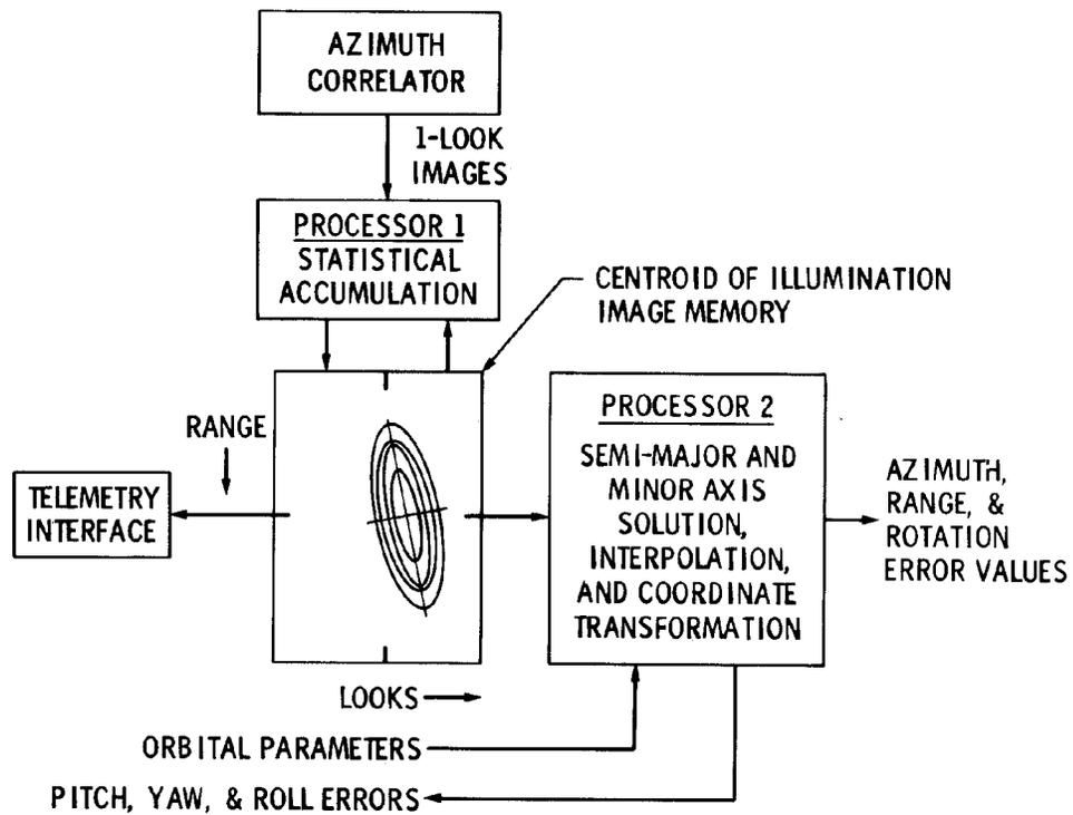
**Figure 8 - SAR Antenna Pointing Error Detector Concept**
