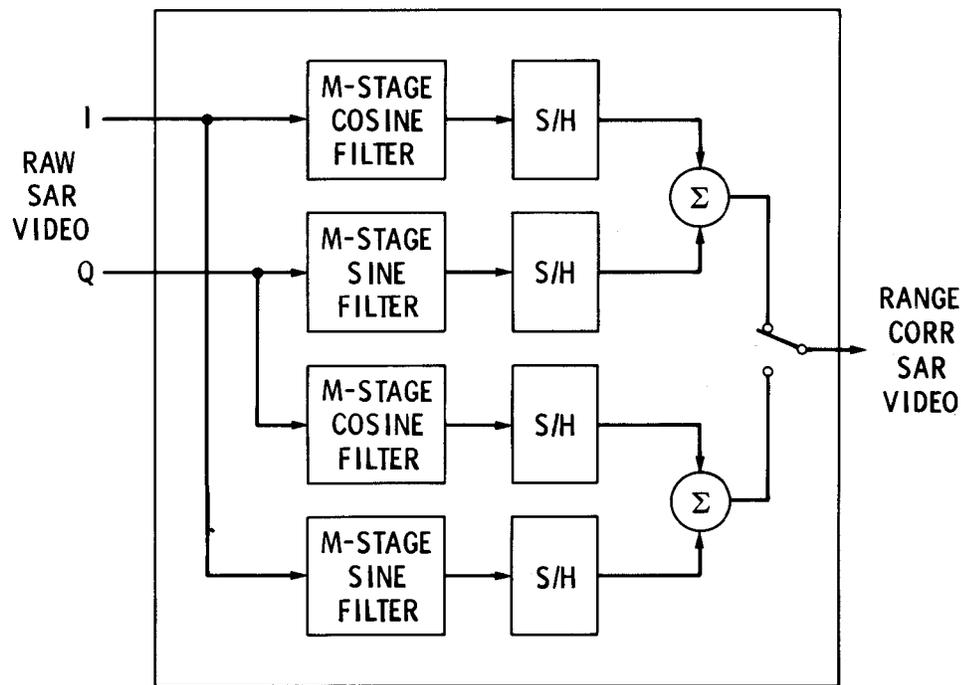
**Figure 2 - Range Correlator Block Diagram**
