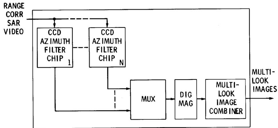
**Figure 4 - Azimuth Correlator Block Diagram.**
