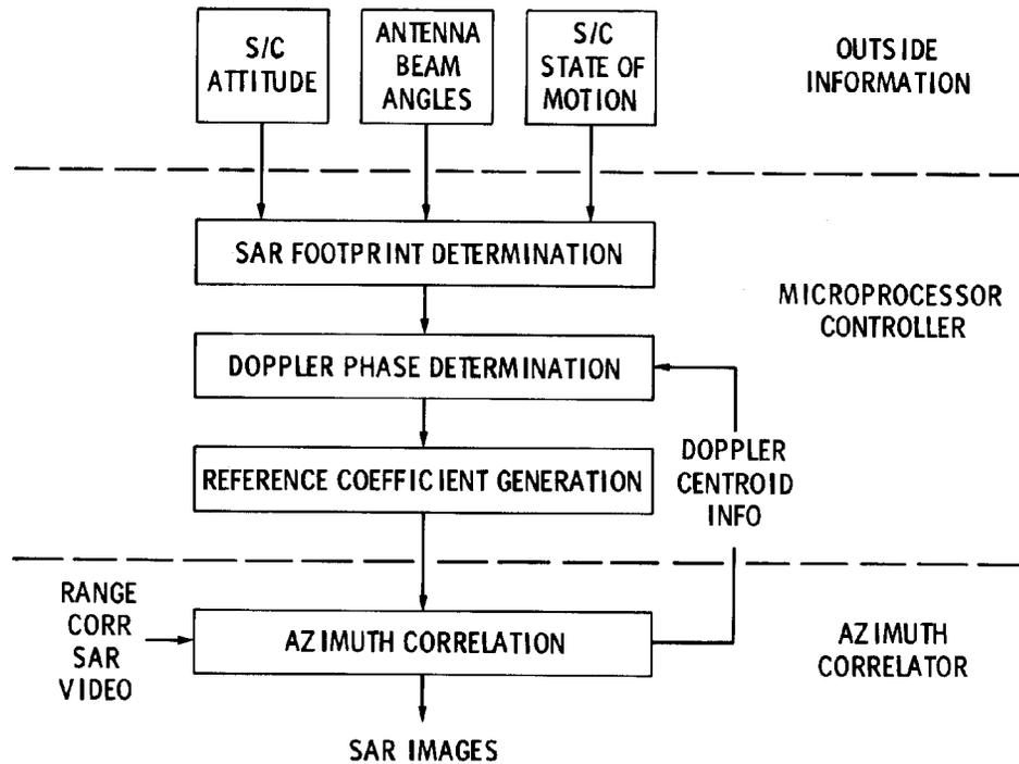
**Figure 6 - Azimuth Reference Function Generation**
