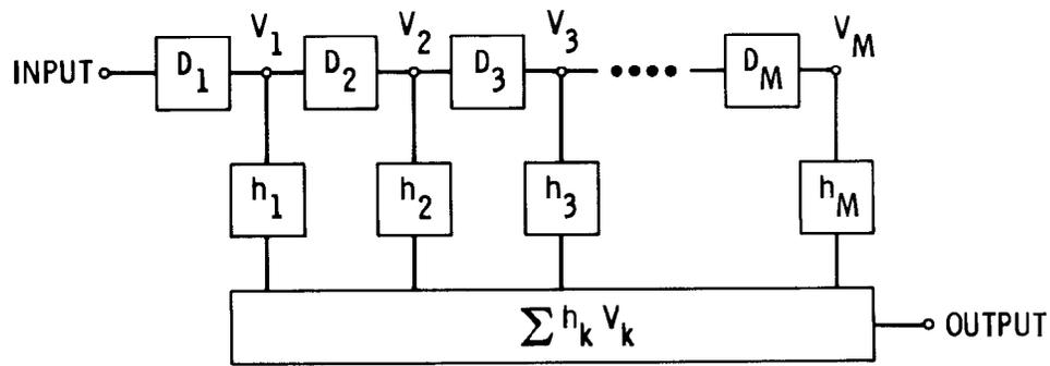
**Figure 3 - CCD Transversal Filter**
