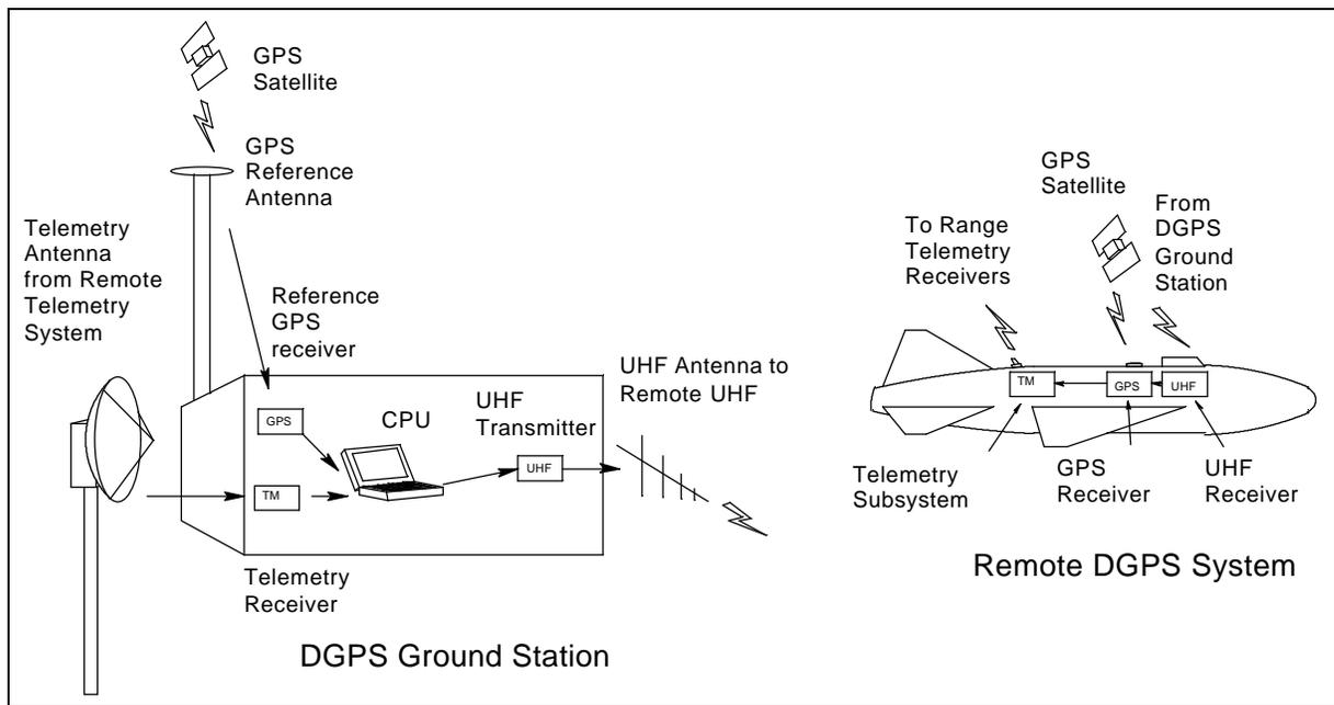
Figure 2. DGPS equipment block diagrams
