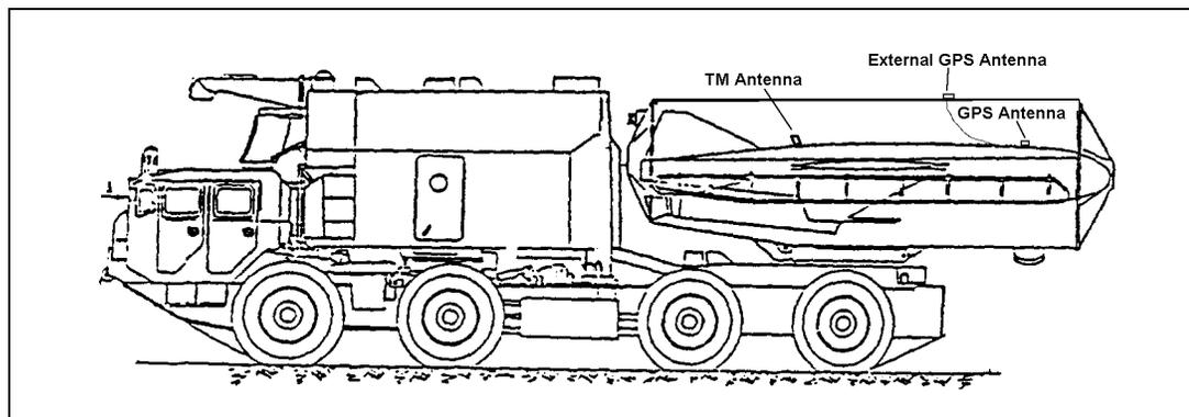
Figure 1. Pre-launch GPS antenna mounting configuration
