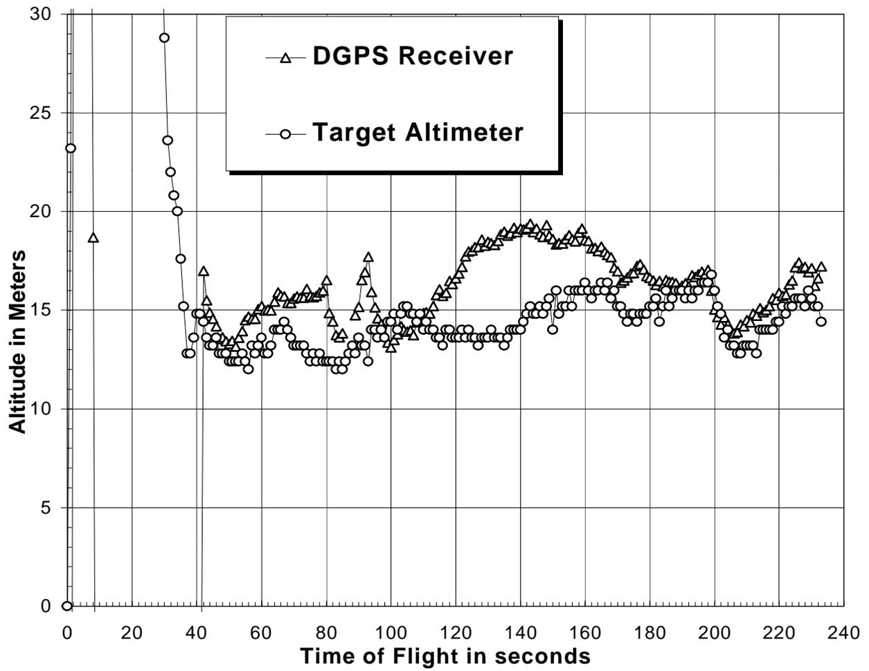
Figure 3. DGPS and altimeter reported altitude
