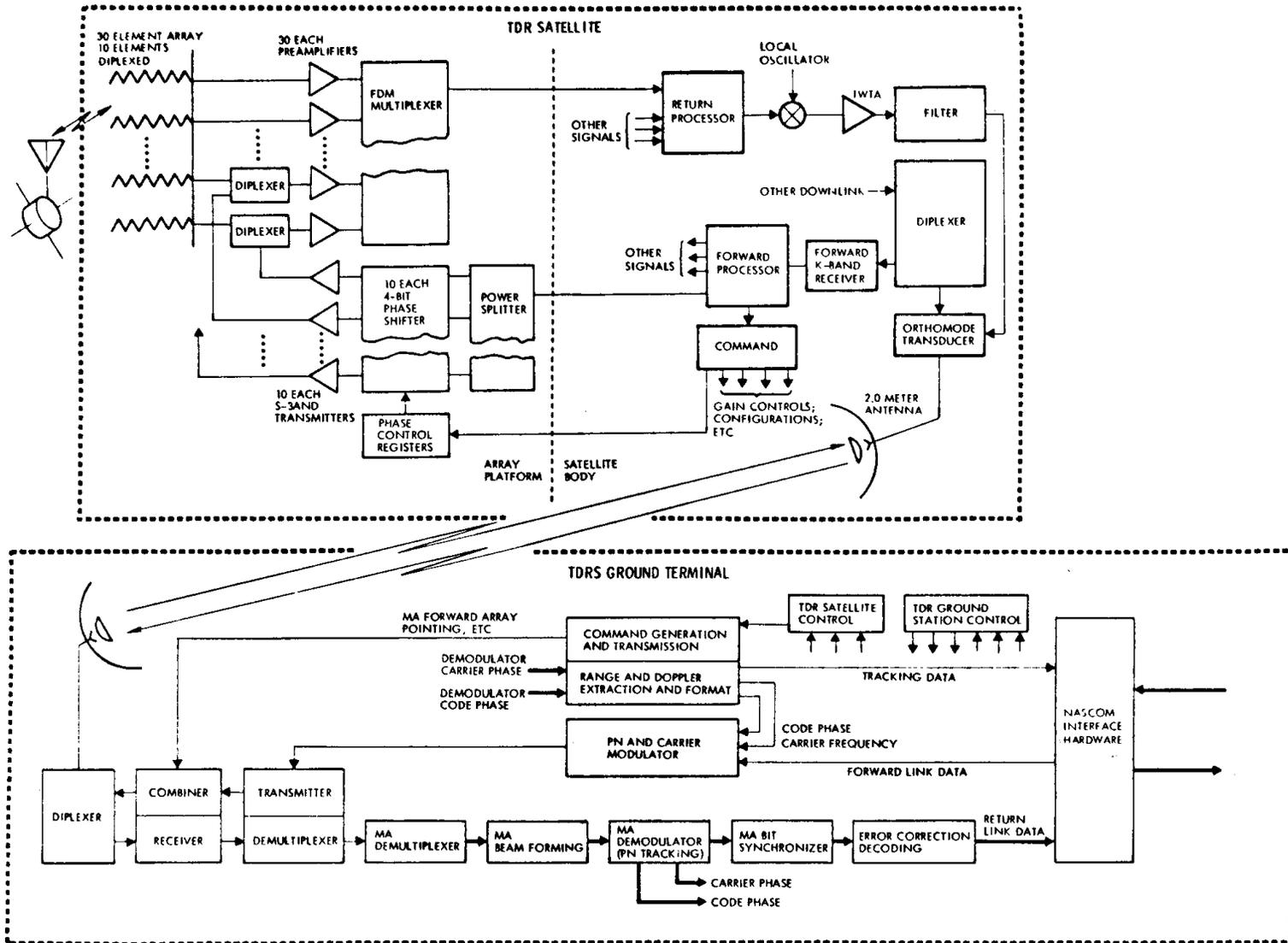
Fig. 2 - MA Link Processing Simplified Block Diagram
